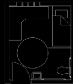
typical accessible inmate cell 1/4" = 1'-0"
