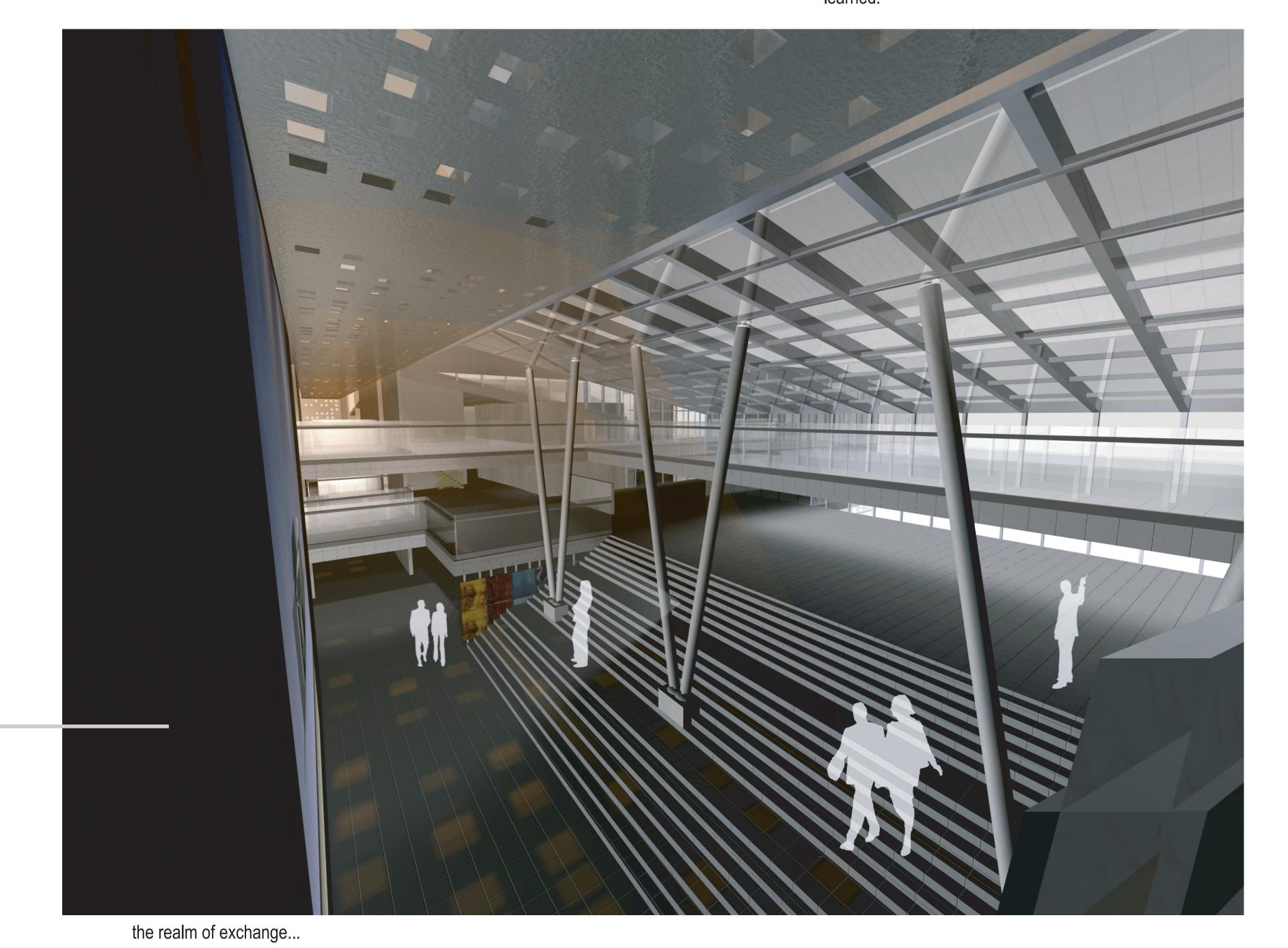
in addition to the broad staircase, a glazed lift, and a media v-shaped columns are stainless-steel ball and socket bearings. the roof construction consists of an orthogonal welded wall, the minimal steel and glass structure of the exchange system of primary and secondary beams that form a rigid center forms a bold contrast to the solid concrete construction of the knowledge area. at the feet of the tubular steel
