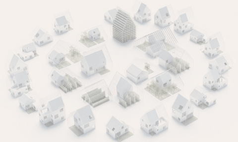
GLASS ENVELOPE THE HOUSING UNITS ARE ENCASED IN A GLASS ENVELOPE TO EXTEND THE GROWING AND LIVING SEASONS IN THE FOOD PRODUCTION FACILITIES AND THE HOUSING UNITS.
