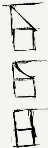
Figure 268—Cell Pod Wall Ceiling Attachment Section Sketches
