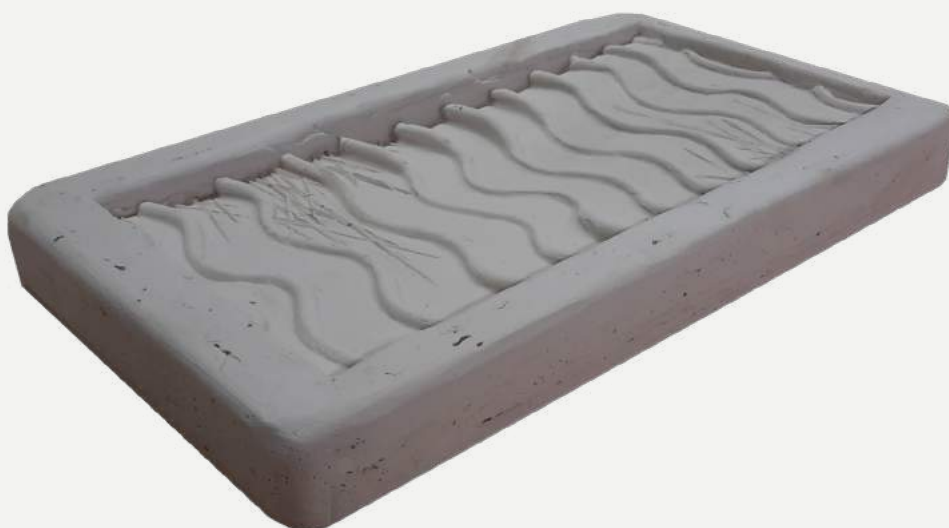
Figure 205 —Wave Tile Plaster Mold
