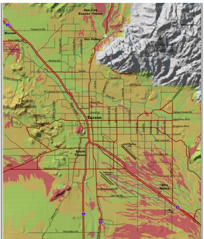
This map shows the shrink/swell potential for the soil in the Tuscon area. Shrink/swelling of the soil is when wind and ephemeral streams deposit loose and under saturated sediments that are prone to collapse.
