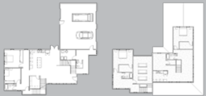
HOUSE 5 ADDITION - LEVEL 1 & 2 FLOOR PLANS
