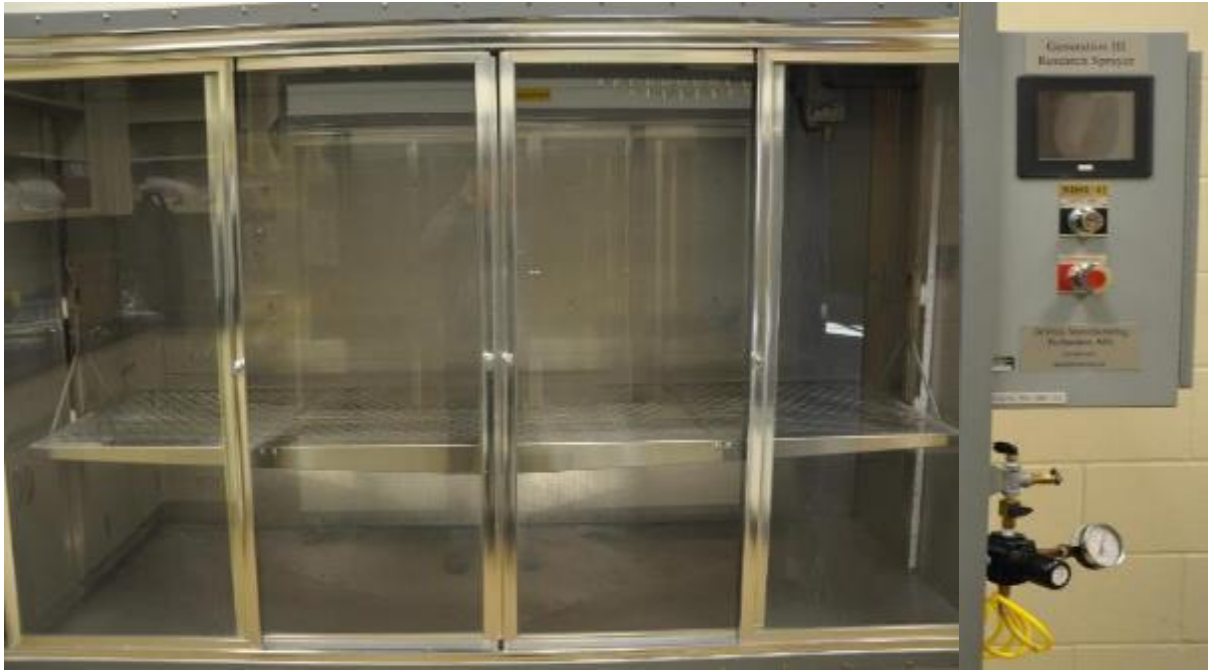
Figure B3. Generation-III Research Sprayer for fungicides adjuvants spray located at NDSU greenhouse.
