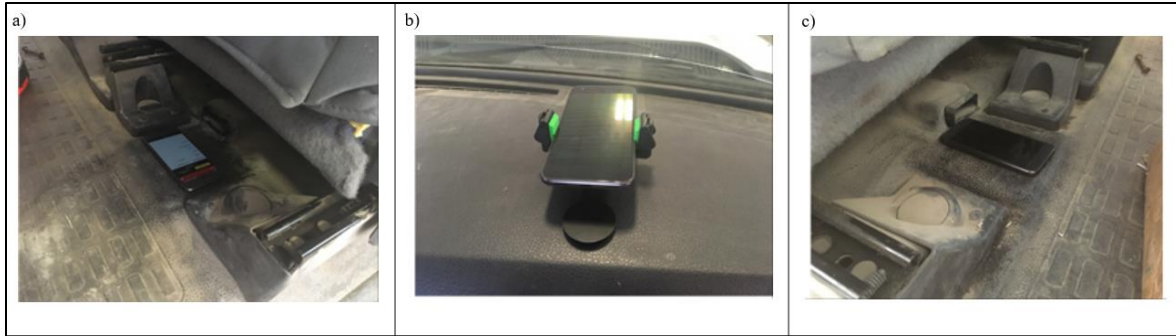
Figure 3.10. a) Phone installed under the passenger seat b) phone installed on the dashboard c) phone installed under the driver seat
