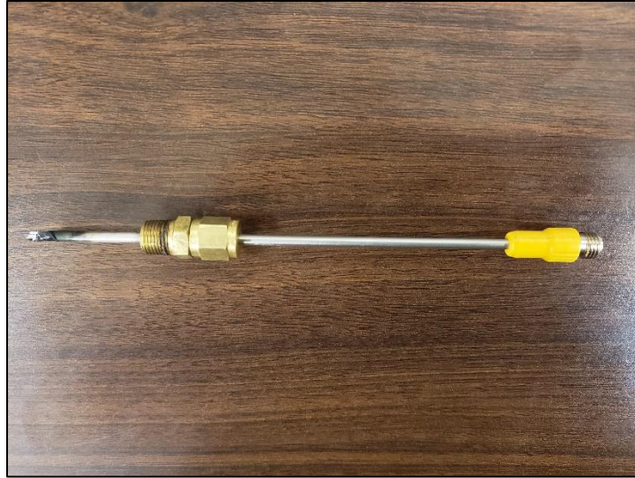
Figure 4.5. Thermocouple Probe After Insertion Into Post-Combustion Region
