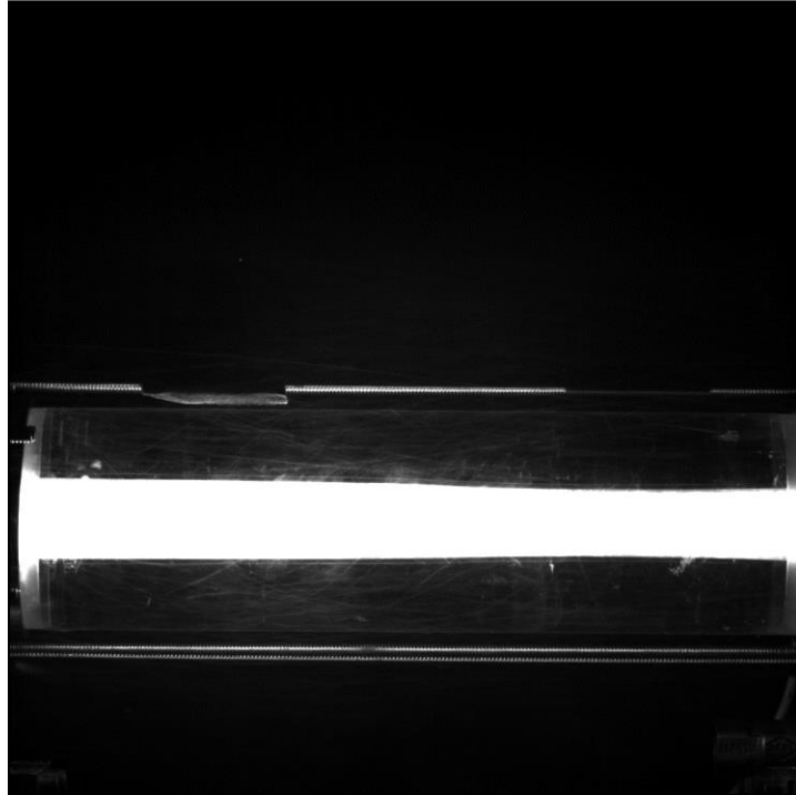
Figure 5.8. Image Taken from High-Speed Recording of Fuel Grain Late in Burn
