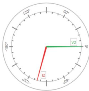
Figure 73. Angular difference between the negative-sequence current and voltage for the synchronous generator.
