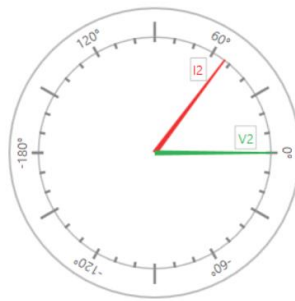
Figure 72. Angular difference between the negative-sequence current and voltage for the solar inverter.
