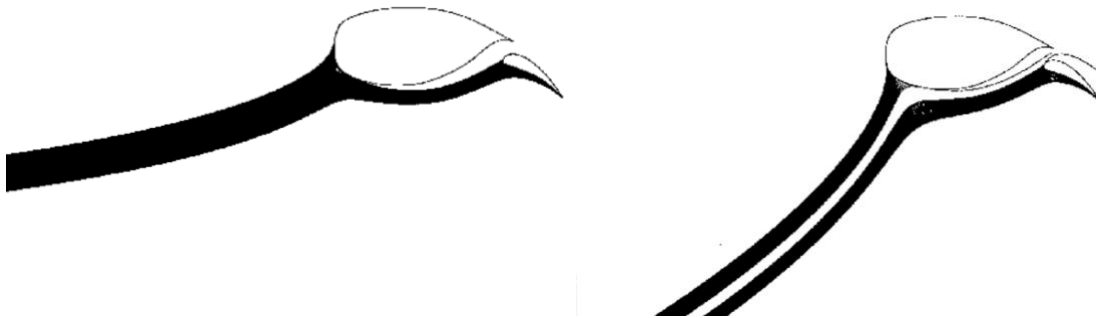
Figure 1.2. Impact angle of droplet on two-element airfoil ( left ): 0^\circ ( right ): 8.1^\circ . Reprinted from reference 25.
