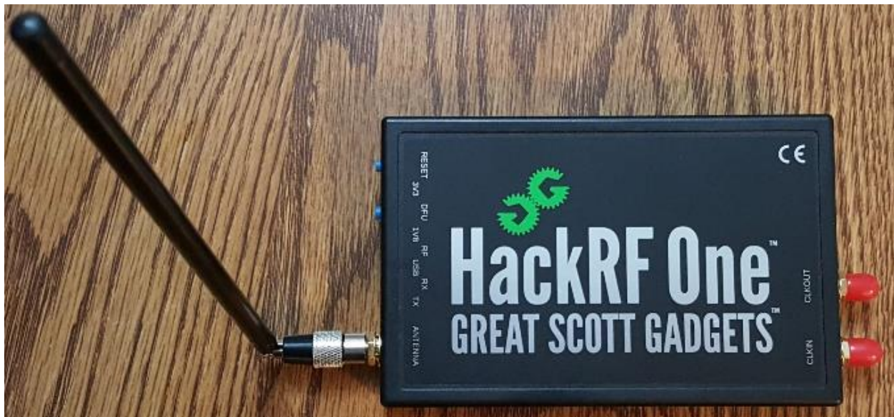
Figure 1. SDR: HackRF One with attached ANT500 antenna.
