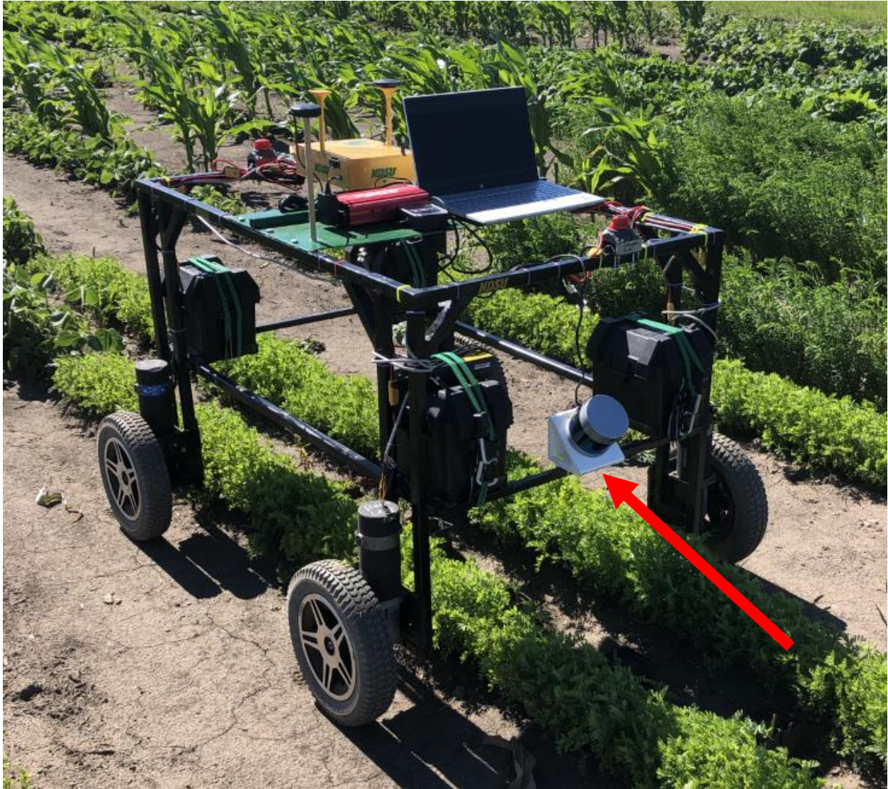
Figure 3.9. Mini Weedbot using a Velodyne VLP-32C LiDAR sensor attached to the front. Built by Dr. Xin Sun's PAG team.
