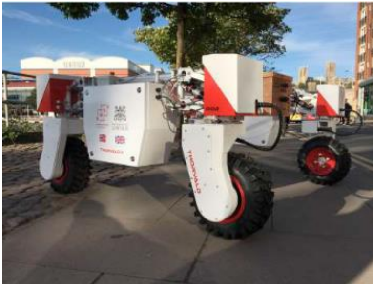
Figure 2.4. Thorvald II robot in standard configuration (Grimstad and From).
