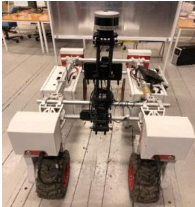
Figure 2.7. Agricultural robot and LiDAR sensor for localization system mapping (Le, et al.).
