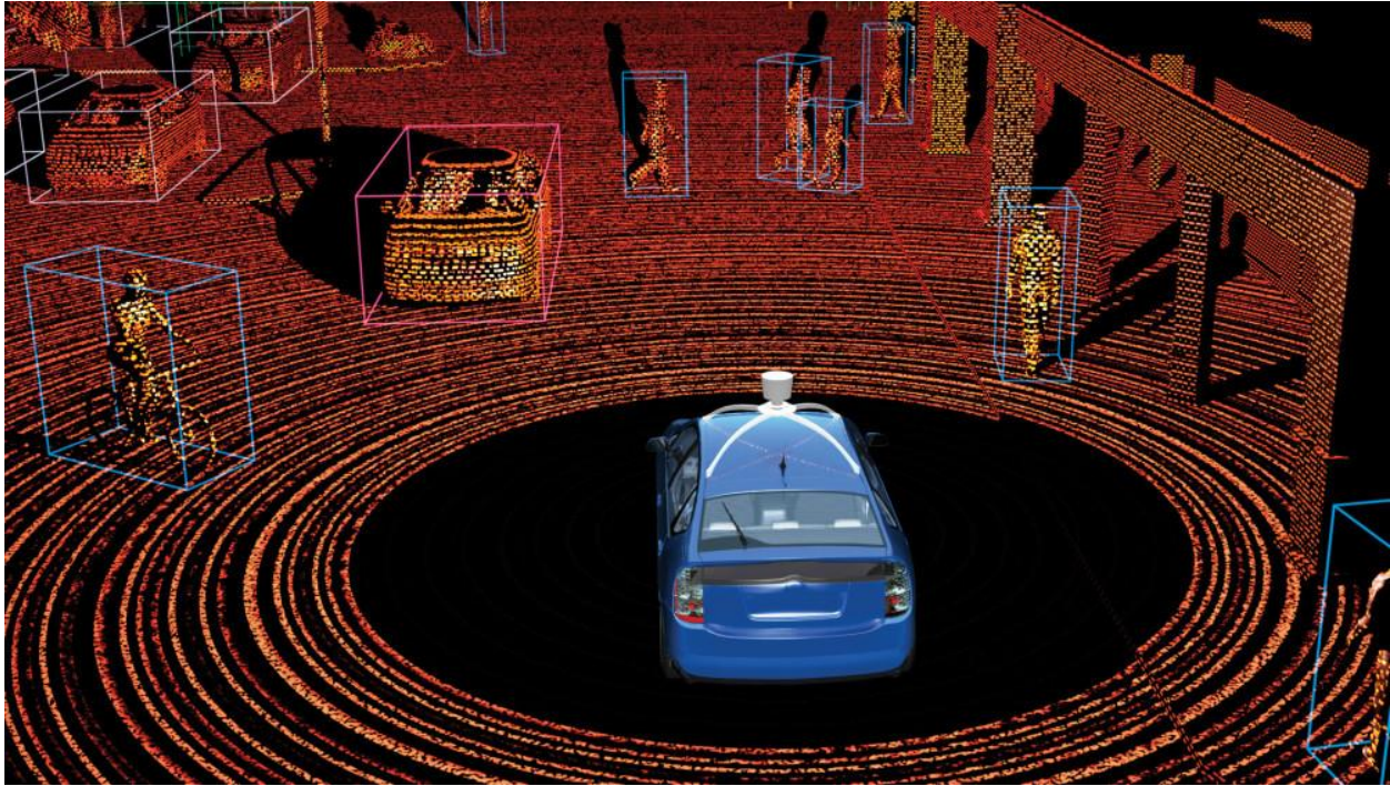
Figure 2.11. Example of LiDAR sensor about of cars surroundings (Allyh).
