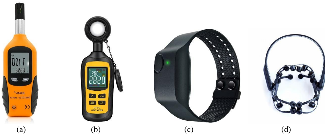
Figure 2: Sensors for data collection (a. Thermal meter b. Illumination meter c. E4 wristband d. EEG headset)
