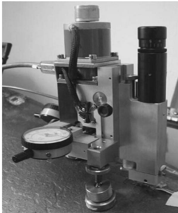
Fig. 2. Incremental hole drilling machine [27].
