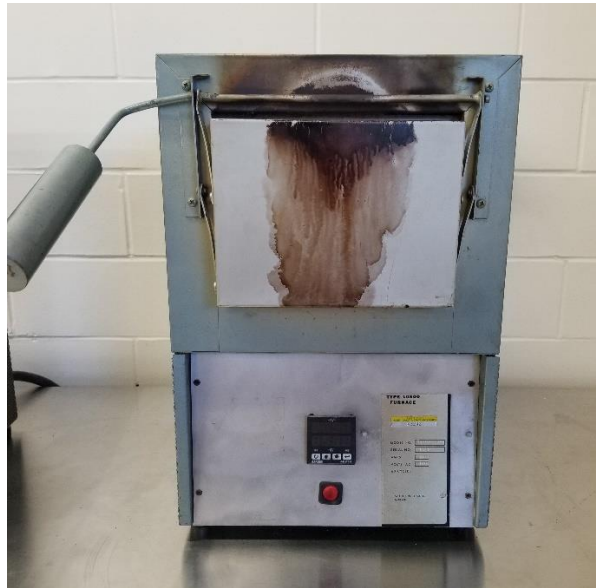
Fig. 10. The furnace used for heat treatment after CS deposition in this study.
