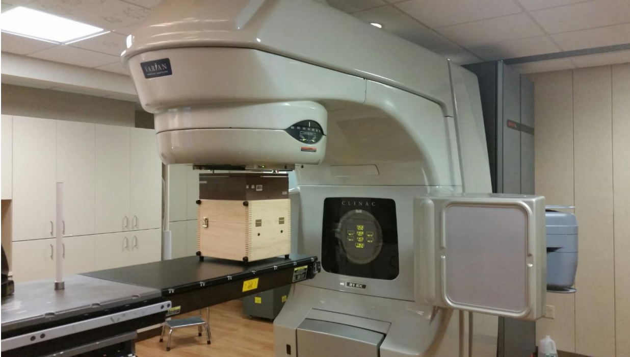
Figure 3: The Varian 21EX linear accelerator used to provide x-ray mutagen dose to sunflower pollen. Located at the Sanford Roger Maris Cancer Center. Sunflower pollen was placed on top of two boxes and beneath a stabilizing plate to ensure proper exposure to high-energy x-rays.
