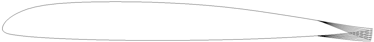
Fig. 2. TE deflection of VR-12 airfoil
