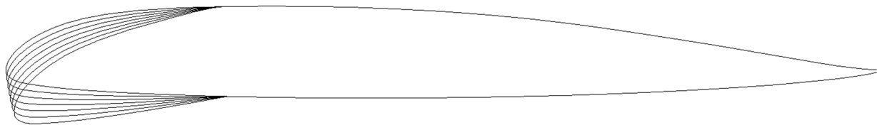
Fig. 3. LE deflection of Boeing VR-12 airfoil
