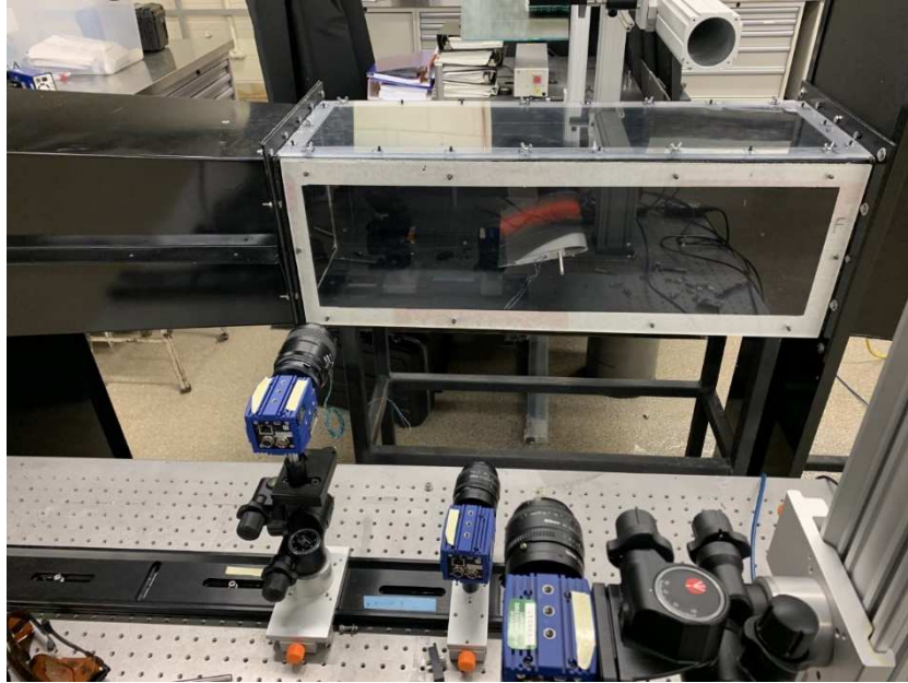
Fig. 10. 2D PIV set up for blower wind tunnel
