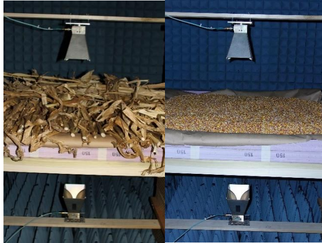
Figure 2. Corn MOG and kernels are shown in the One Meter Fixture.
