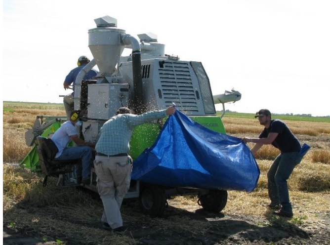
Figure 13. A tarp is used to capture wheat residual material as it is discharged from the rear of a plot combine.
