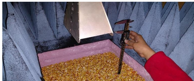
Figure 11. A caliper's depth rod is used to verify uniform material depth (thickness) within the fixture.
