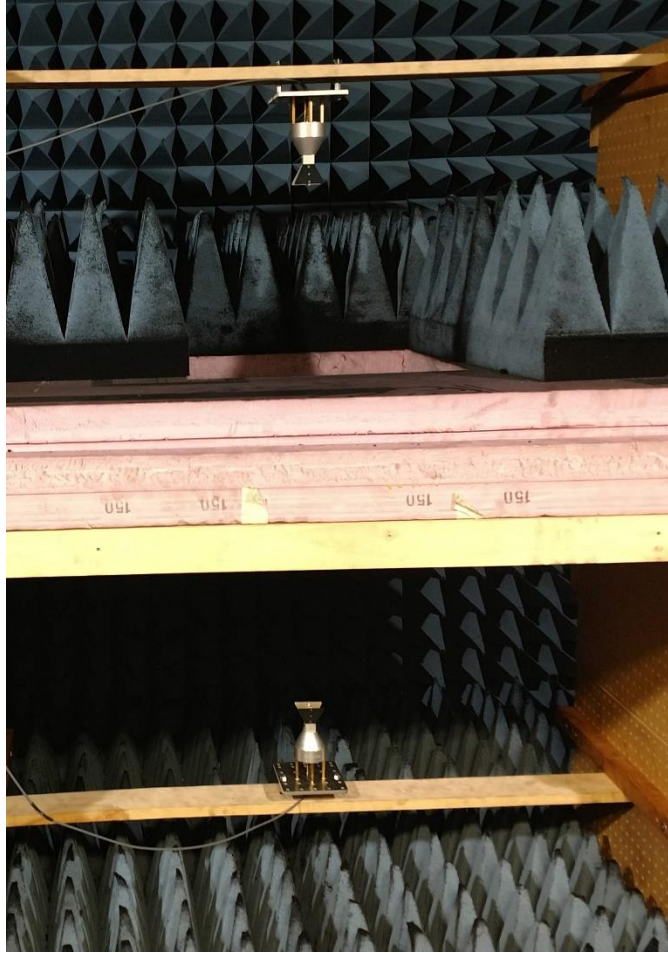
Figure 7. The Reduced Fixture is shown with MVG SH5000 (5-50 GHz) antennas installed. In this photo, the antennas are shown with 109 mm antenna-to-antenna spacing.
