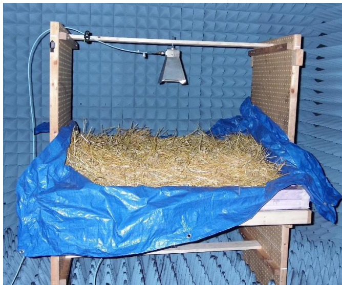
Figure 14. Wheat MOG (combine residue) is shown in the One Meter Fixture.
