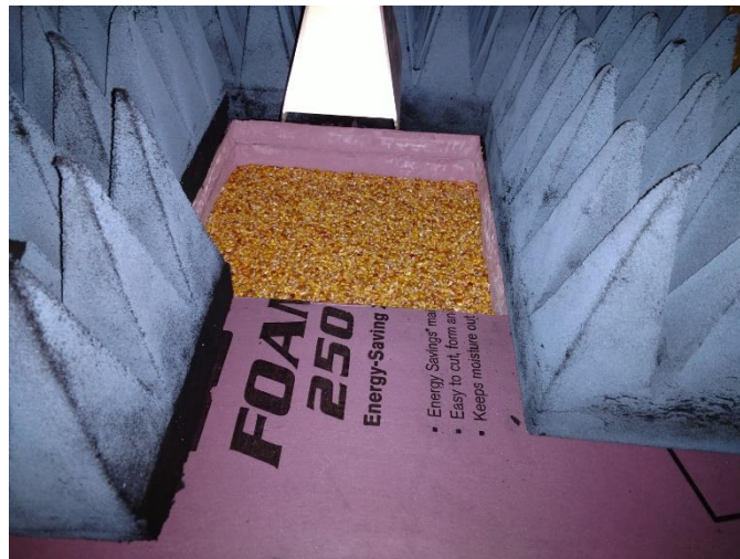
Figure 4. Corn kernels are shown in the Reduced Fixture. Anechoic foam absorbers surround the sample space; note that one absorber has been removed for this photo so that the grain sample can be seen.
