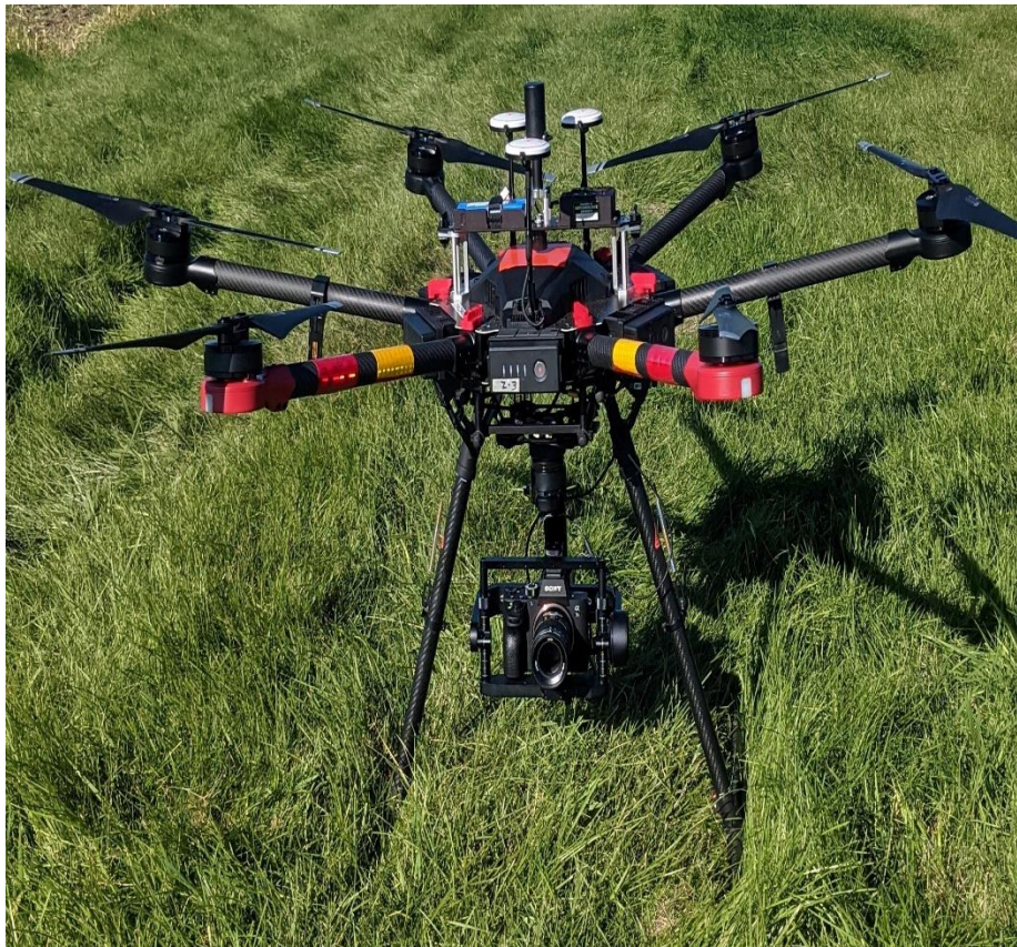
Figure 2. DJI Matrice 600 Pro with a Sony Alpha 7R II, 42.4-megapixel RGB camera mounted on it. The drone is loaded with 6 batteries and a Geosnap PPK system is integrated to the UAS by mounting it on the top part of drone.
