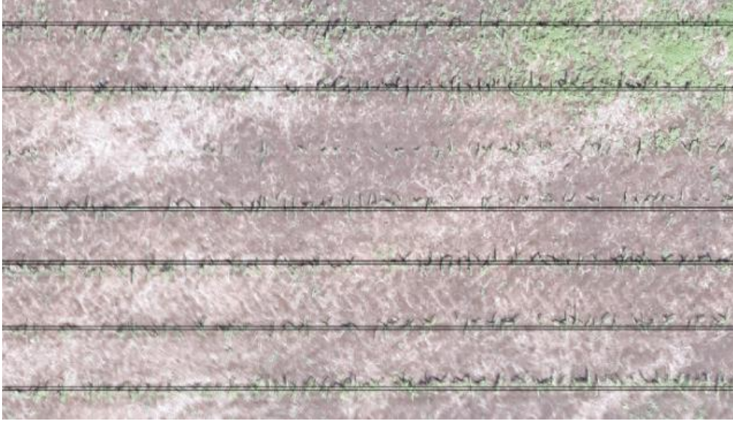
Figure 12. Sample image where the proposed PIP algorithm failed to detect an existent corn row as a line on the ExGI imagery of a corn. Imagery captured by Sony Alpha 7R II, flown at 350 ft AGL.
