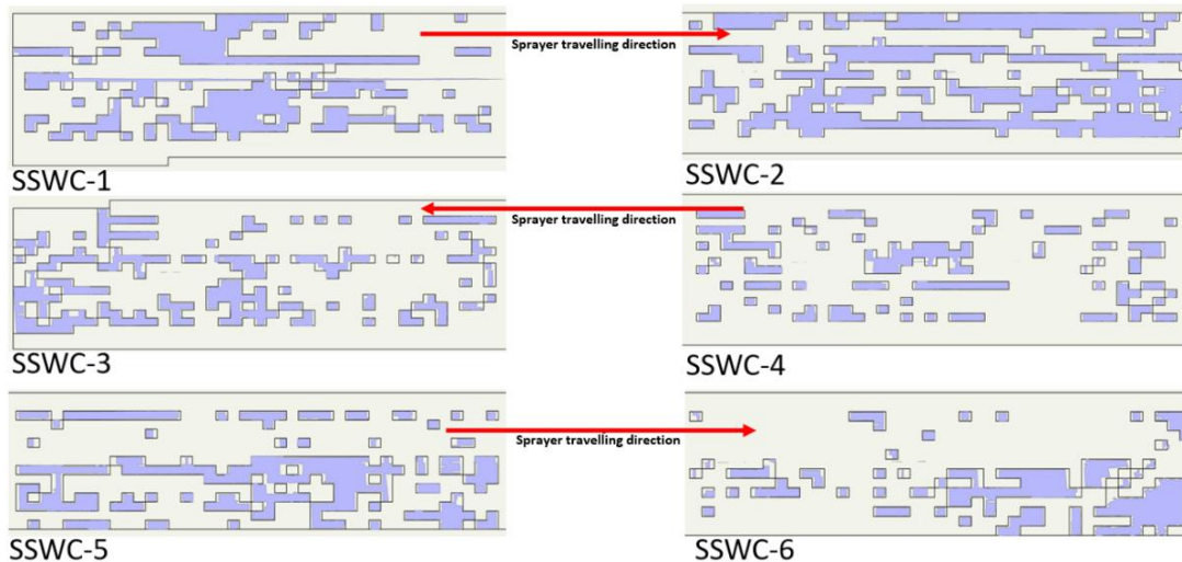
Figure 15. Overlap of Rx map, generated by AgSMS, where the regions enclosed by dark black lines where the no-spray regions (0 gal/ac), and the as-applied map. Purple color regions are the area where the sprayer turned its nozzles off while operating at 6.5 mph speed (approximate), while all the remaining area was sprayed (15 gal/ac).
