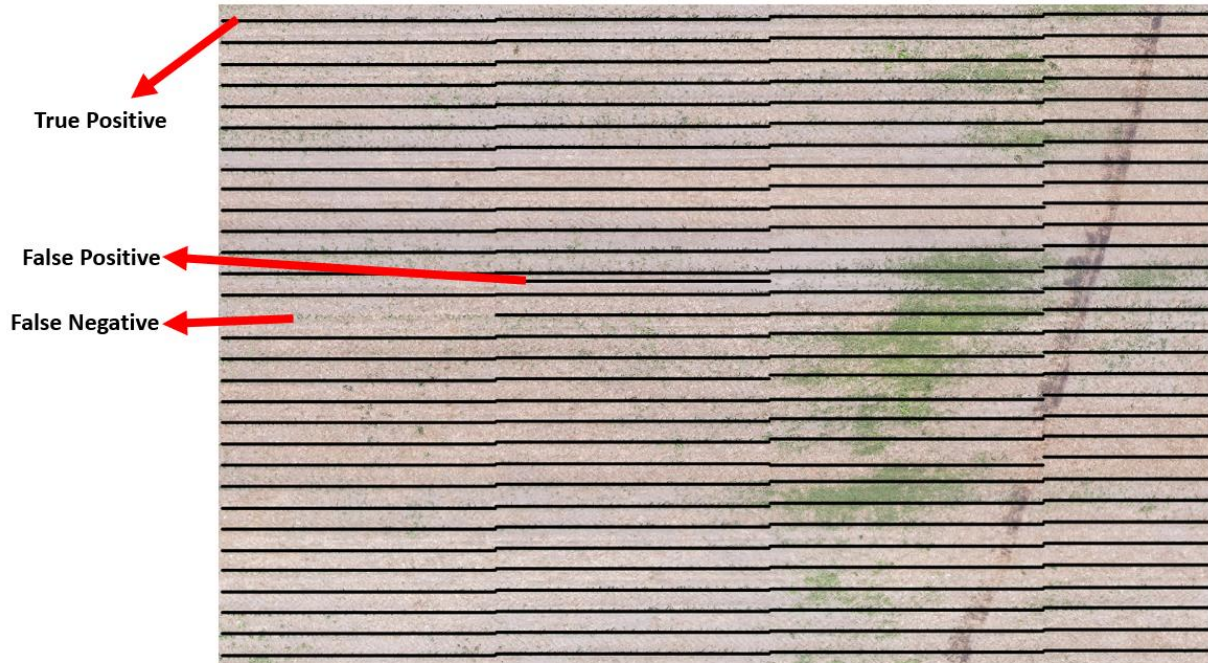
Figure 11. Comparison of actual corn rows with the identified lines created by the Pixel Intensity Projection algorithm on a corn field imagery captured by Sony Alpha 7R II, flown at 350 ft AGL
