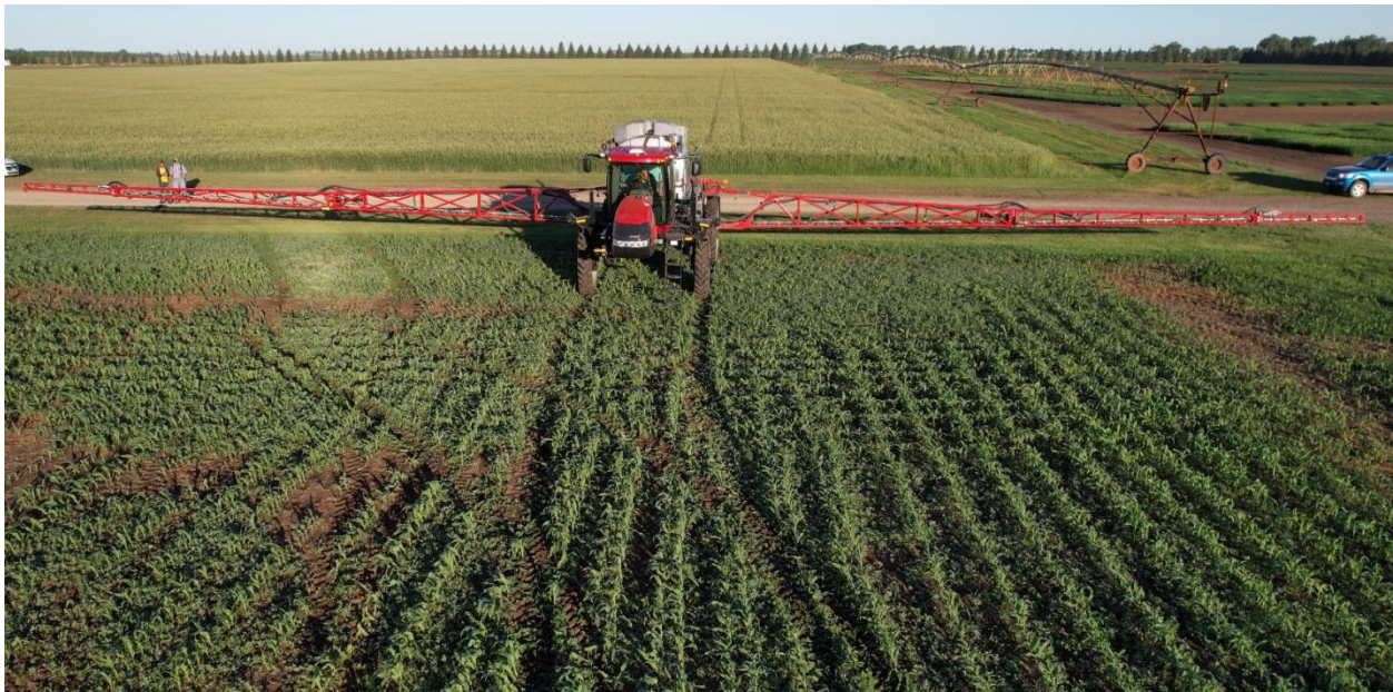
Figure 9. Case IH Patriot 4440 series sprayer used to implement site-specific weed control in a corn field. The sprayer was equipped with an AIM command FLEX system, RTK GPS receiver, Viper 4+ cab computer, and 136.6 ft wide boom
