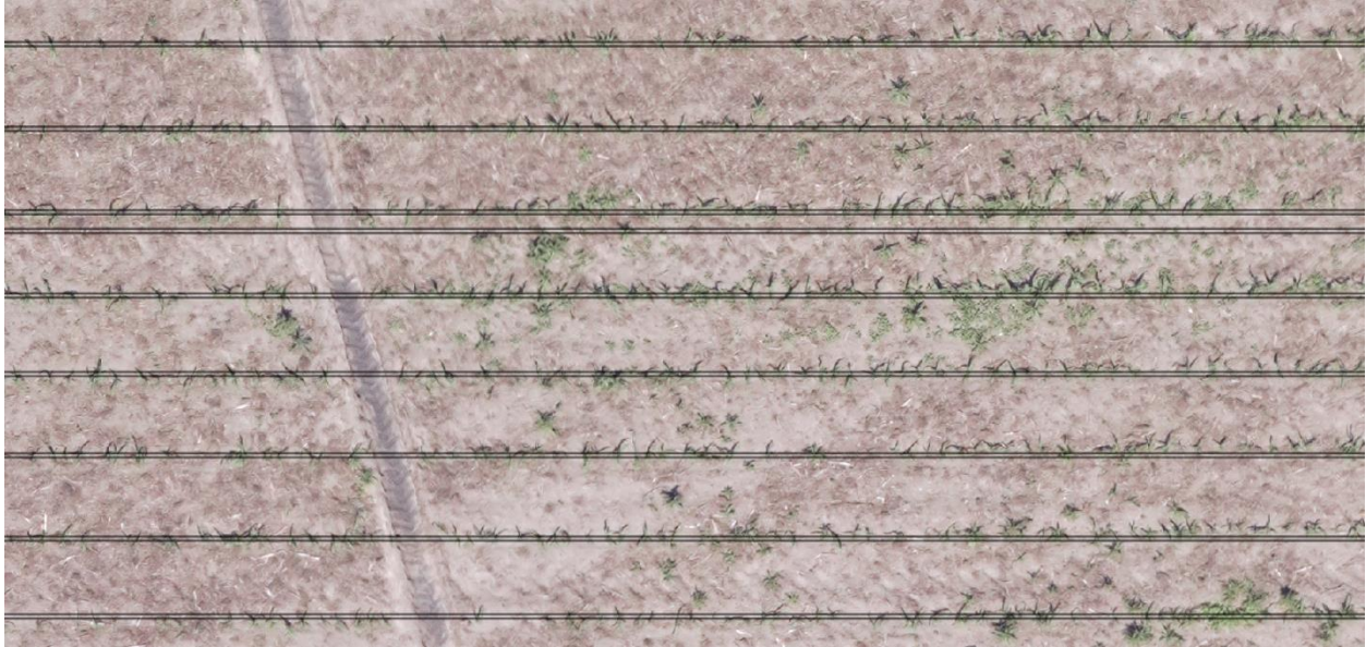
Figure 13. Sample image where the proposed PIP algorithm detected two lines over a single corn row on the ExGI imagery of a corn field. Imagery captured by Sony Alpha 7R II, flown at 350 ft AGL.
