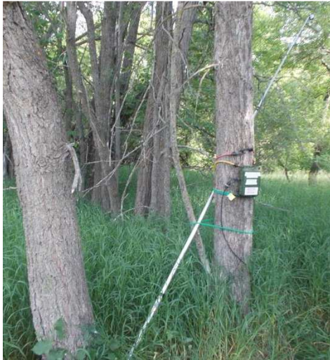
Figure 2. Stationary monitoring setup at a typical site. The SM4BATFS acoustic bat detector is strapped to the tree, while a Wildlife Acoustics U2 microphone is attached to the end of the extendable flagpole (silver color)
