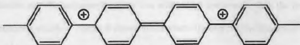
Figure 7: Bipolaron in a nondegenerate polymer (Roth & Carroll, 2004).
