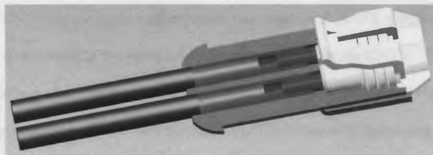
Figure 50: Cut away view of female connector with inserted male connector.
