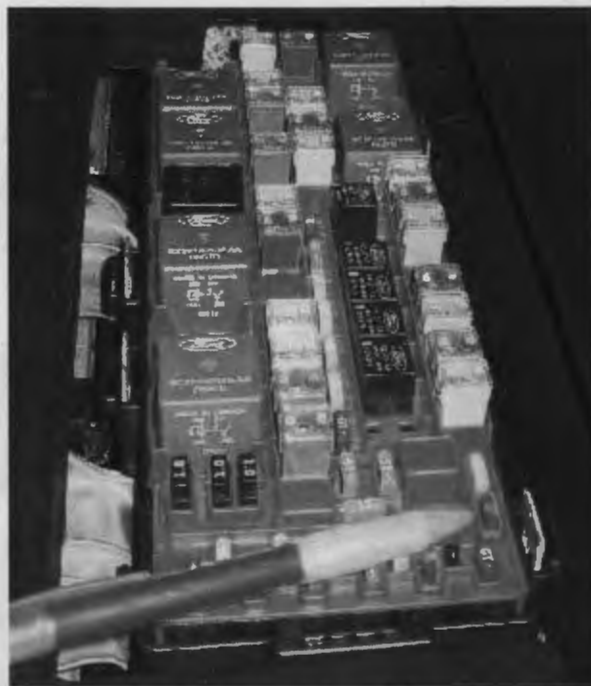
Figure 46: Typical fuse relay center.
