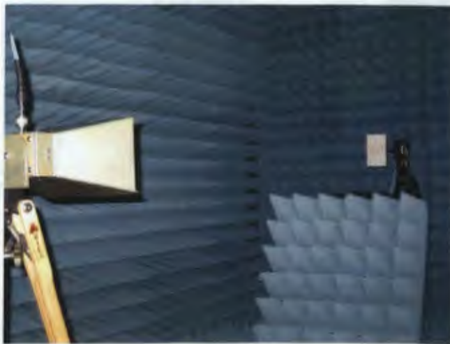
Figure 19. Measuring the radiation pattern in the x-z plane in an anechoic chamber.
