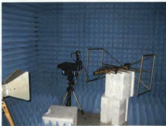
Figure 22. Gain measurement setup with reference biological antenna in an anechoic chamber.
