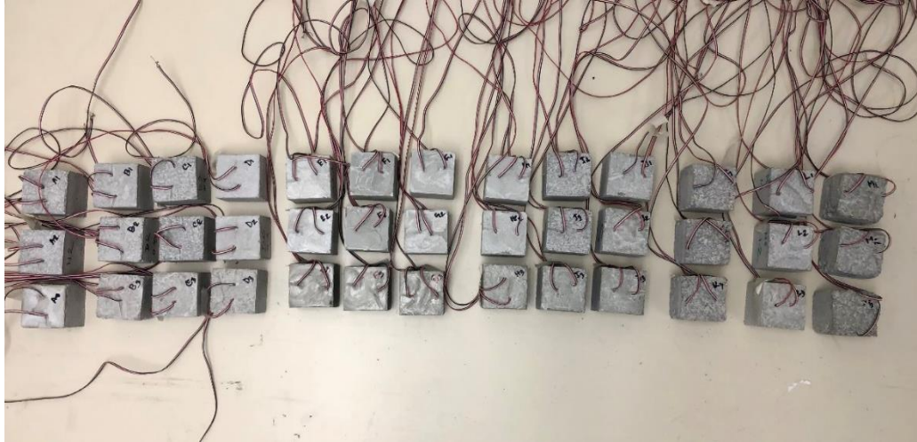
Figure 8. The sample groups from three different dispersion methods with different water-cement ratios.
