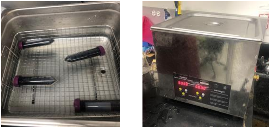
Figure 5. The test tubes with carbon nanotubes with NaDDBS being placed in the sonicator.
