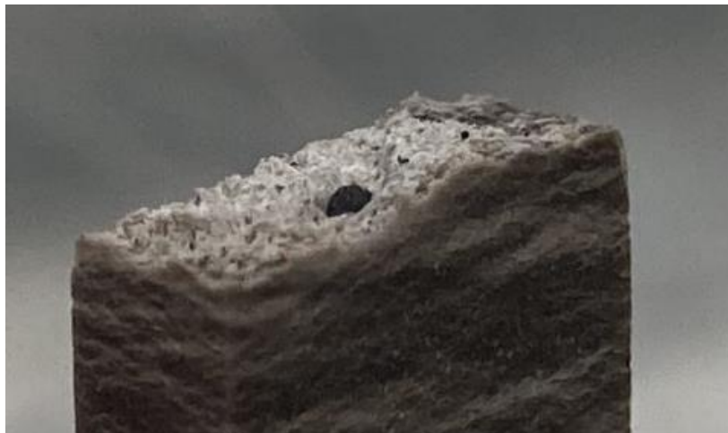
Figure 35. Injection Molded MSC-40C Tested Tensile Specimen Fracture Surface View Three
