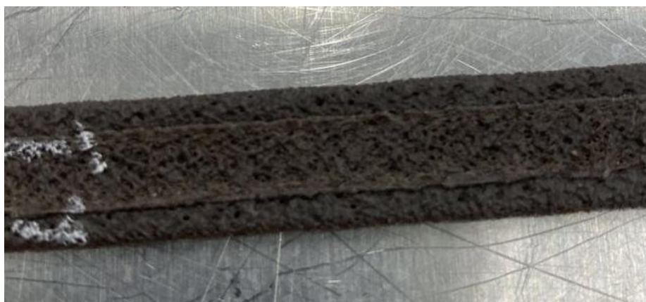
Figure 32. Additive Manufacture MSC-40C Part Surface Finish Example
