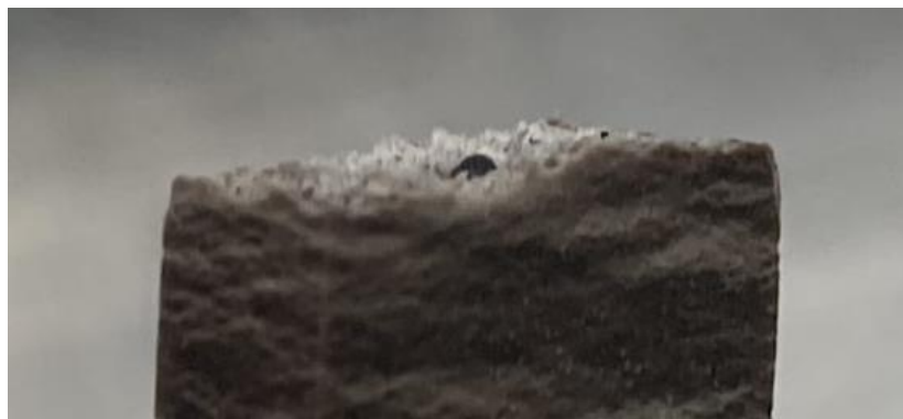
Figure 34. Injection Molded MSC-40C Tested Tensile Fracture Surface View Two
