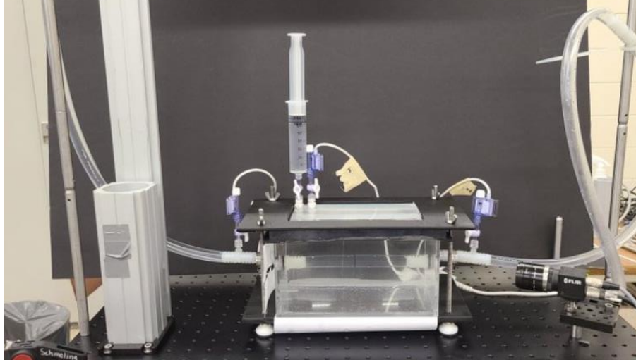
Figure 14. Experimental setup for establish the local tube law.
