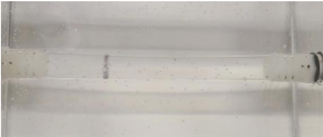
Figure 21. Circle drawn on tube for steady flow experiments. The circle is shifted downstream of the center of the vessel.
