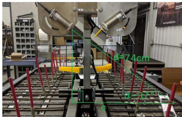
Figure 3.7. Adjusted angle of ultrasonic sensor to emit the sound frequency.
