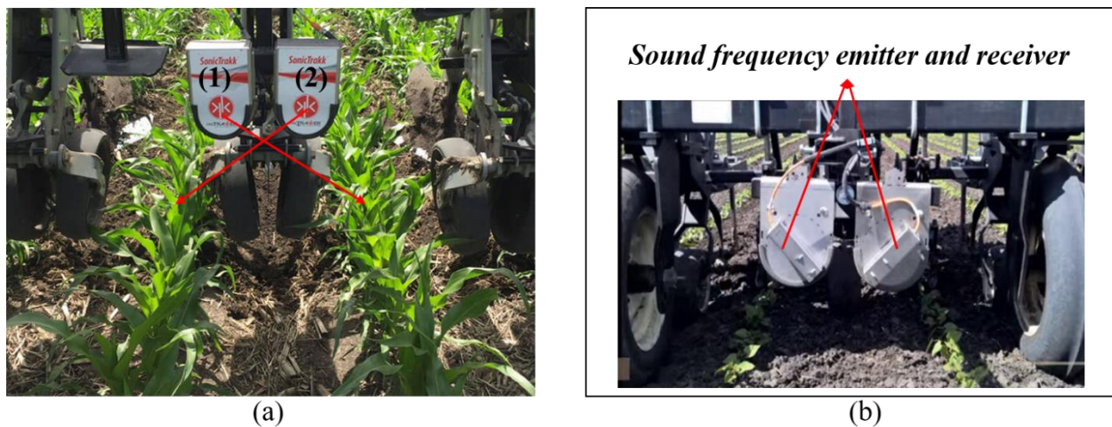
Figure 3.2. Ultrasonic sensor for measuring the distance to the plants.
