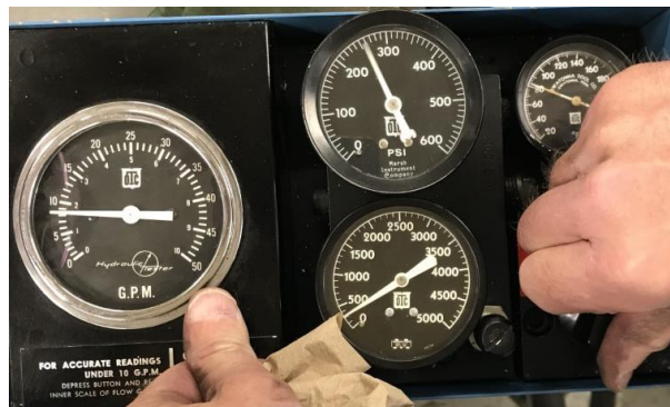
Figure 5.5. Flowrate measurement of the hydraulic power pack.
