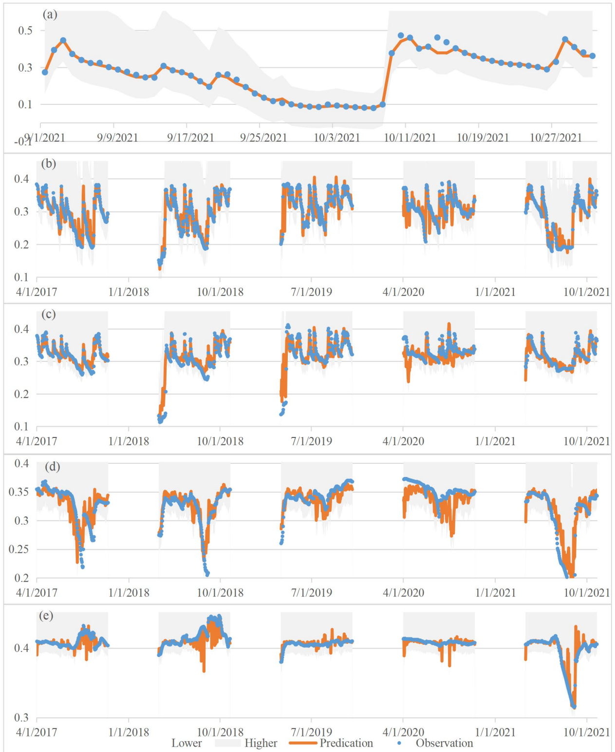
Figure B11. Graphical comparison of observed (blue dots) and GPR-simulated (orange lines) soil moisture at 5 cm (a), 10 cm (b), 20 cm (c), 50 cm (d), and 100 cm (e) in Waukon. Notes: (1) GPR – Gaussian Process Regression. (2) The shaded areas are 95% confidence region.
