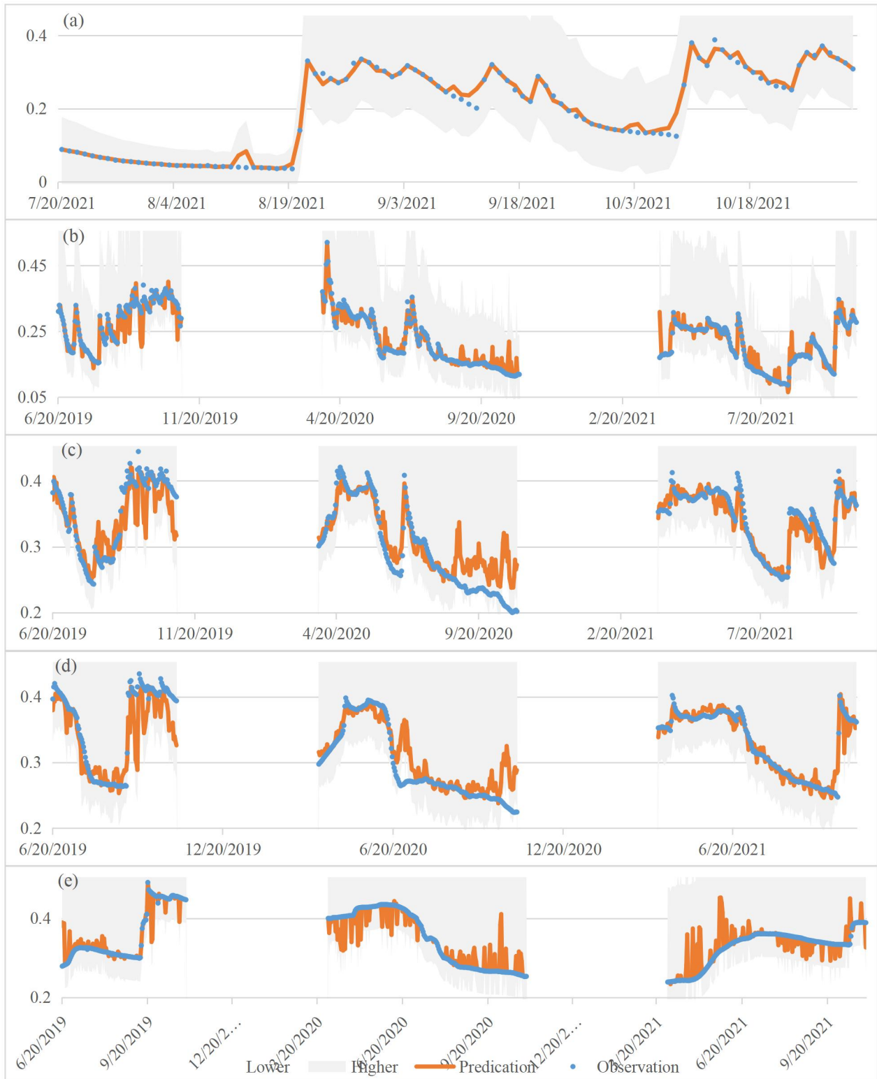
Figure B19. Graphical comparison of observed (blue dots) and GPR-simulated (orange lines) soil moisture at 5 cm (a), 10 cm (b), 20 cm (c), 50 cm (d), and 100 cm (e) in Denhoff. Notes: (1) GPR – Gaussian Process Regression. (2) The shaded areas are 95% confidence region.
