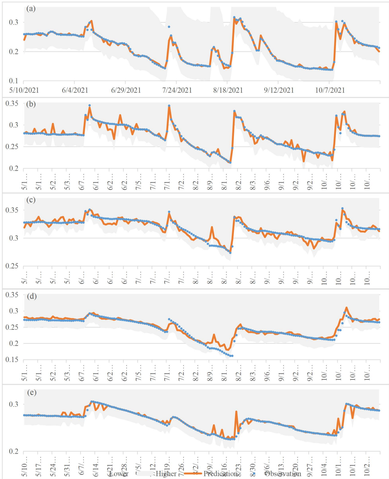
Figure B26. Graphical comparison of observed (blue dots) and GPR-simulated (orange lines) soil moisture at 5 cm (a), 10 cm (b), 20 cm (c), 50 cm (d), and 100 cm (e) in Perth. Notes: (1) GPR – Gaussian Process Regression. (2) The shaded areas are 95% confidence region.
