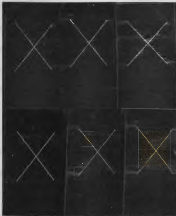
Figure 4.21. The visual evaluation of the sulfate doped PPY/Al Flake coated panels (top) and the vanadate doped PPY /Al Flake coated panels (bottom) at 72, 216, and 552 hours of B117 exposure.
