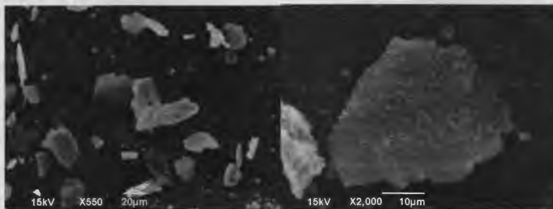
Figure 3.22. SEM micrographs of the flake synthesized in the presence of vanadate.
