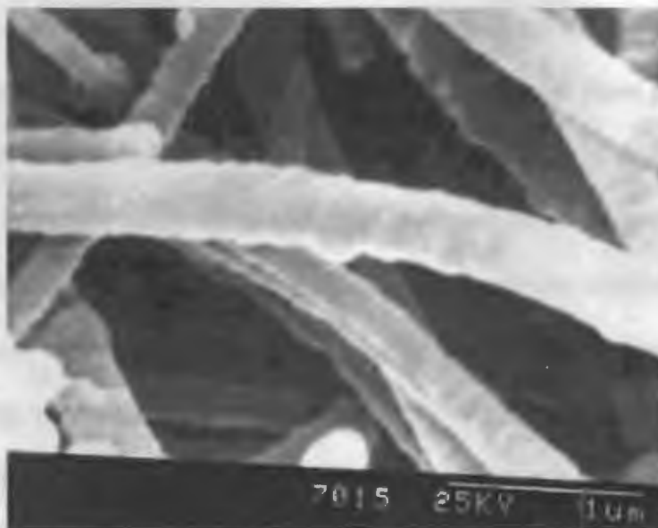
Figure 1.17. Fibrils of polypyrrole doped with \beta -naphthalene sulphonic acid.[57]
