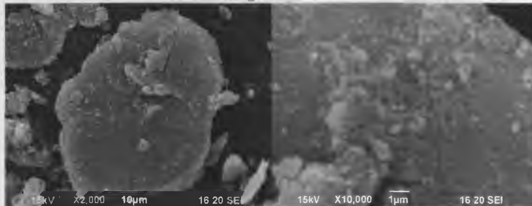
Figure 3.8. SEM micrographs of ground product from reaction 5, 10 \mu\text{m} (left) and 1 \mu\text{m} (right).
