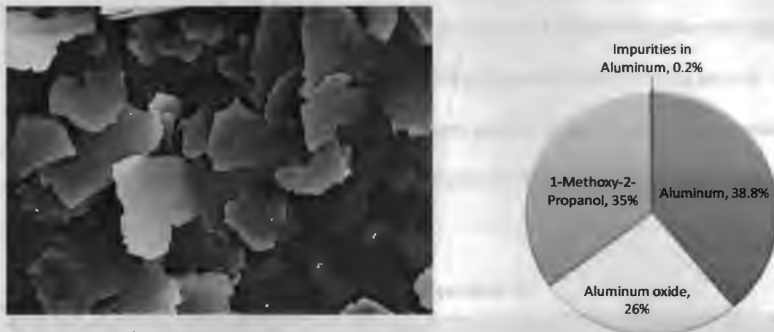
Figure 3.1. SEM micrograph of the as-received aluminum flake (left) and the composition by weight (from MSDS) (right).
