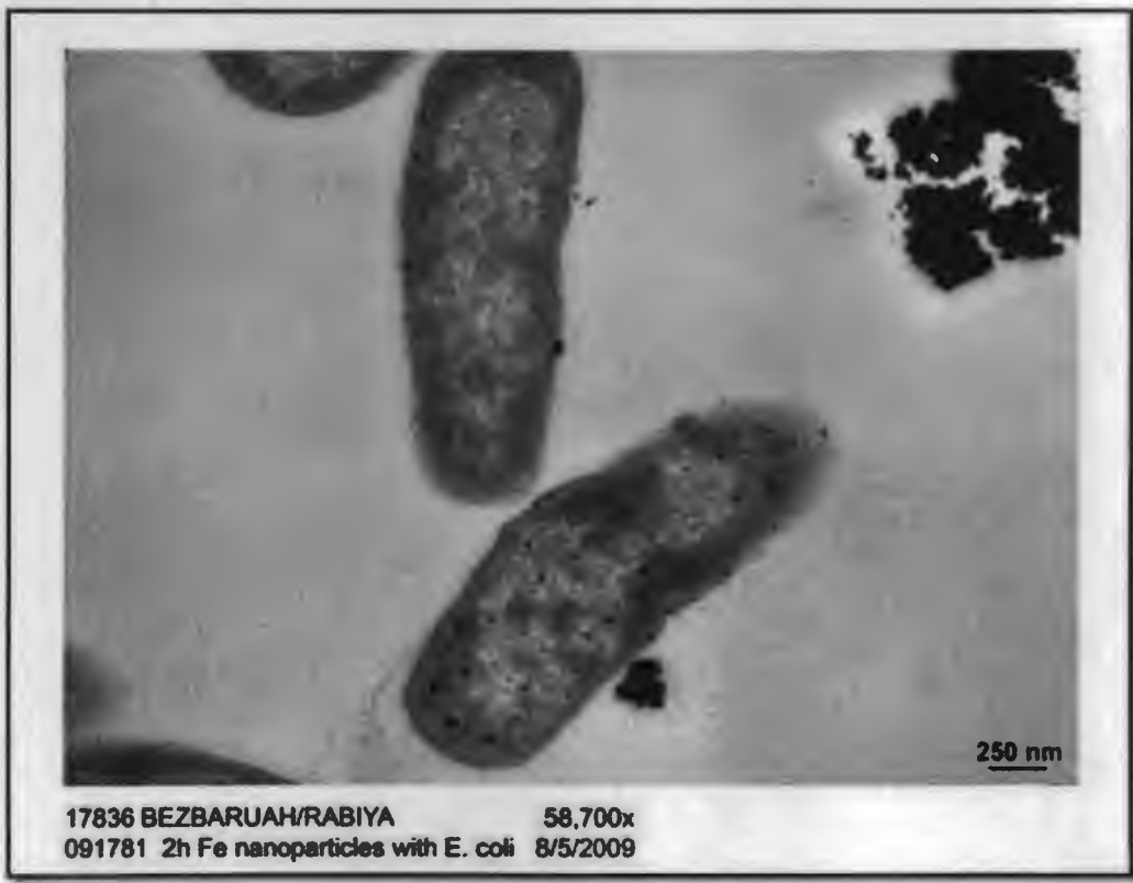
Figure 3.16: TEM images do not give clear idea about the location of NZVI. While the cell on the bottom shows that particles are inside. However, these are two dimensional sections and it is difficult to infer whether the particles are outside or inside the cells.
