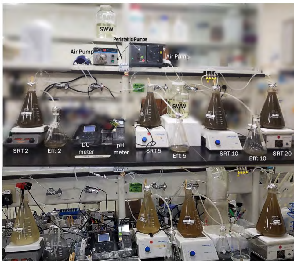
Figure 3.1. Bench-scale experimental setup for chemostat operation on day 1 (top) and day 20 (bottom). SWW – synthetic wastewater water; Eff – effluent; SRT – solids retention time.
