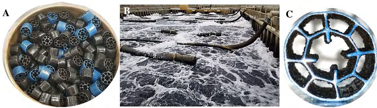
Figure 4.1. Biofilm carriers (A) collected from MBBR basin (B), magnified image of a single biofilm carrier with accumulated biofilm inside (C).
