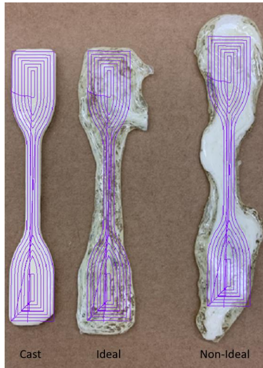
Figure 15. PX printed specimens with highlighted print path imposed on the photo.
