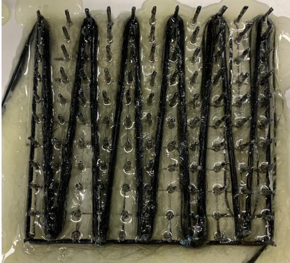
Figure 30. Uniform z fiber reinforced bed with continuous carbon fiber printed on top.
