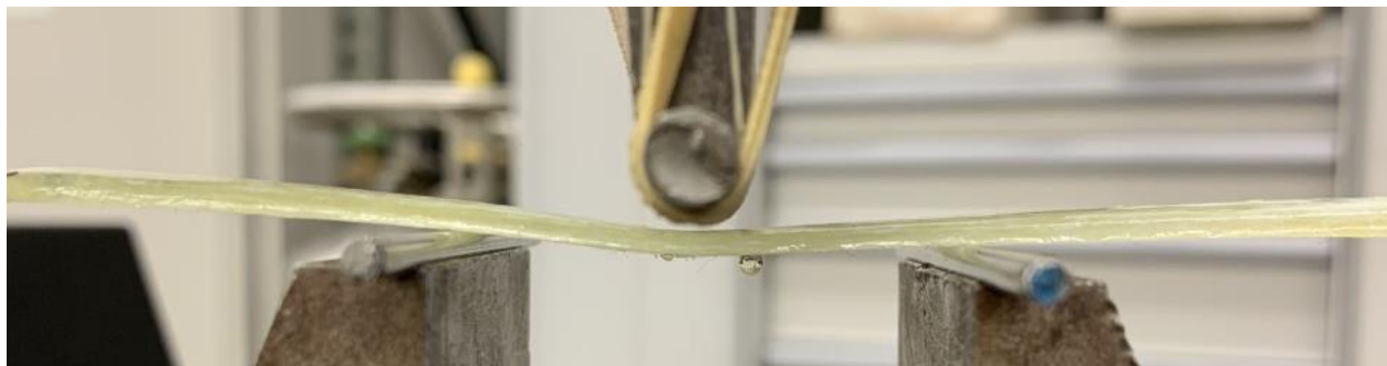
Figure 24. PX flexural specimen leaking pentaerythritol resin.
