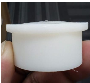
Figure 25. Dome-shaped protrusion on 100% PBS cup
