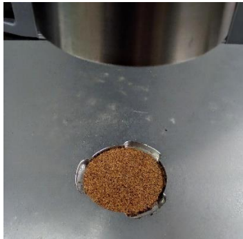
Figure 26. Cork-padding in fixture cavity to prevent rotation of parts
