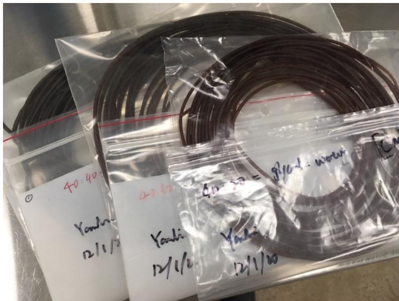
Figure 6.1. Extruded filament for 3D printing.
