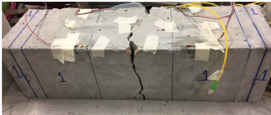
Figure 19. Comparison of Detected Crack Compared with Reference Crack (a) and Photo of after Cracking (b) for Sample 1
