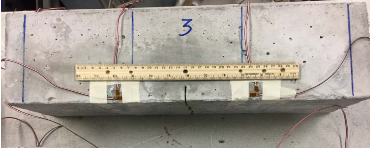
(a) Concrete beam sample with initial notch 75mm
