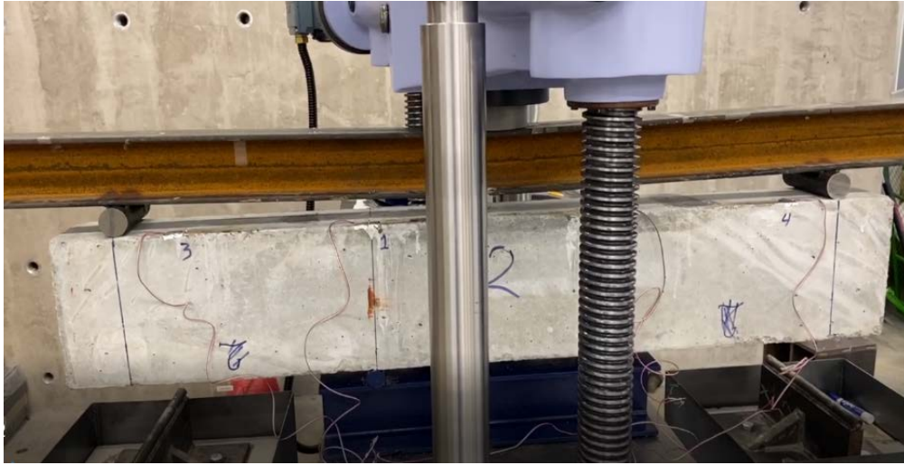
Figure 27. Front View of the Loading Arrangement and the RC Beam Instrumented with Sensors
