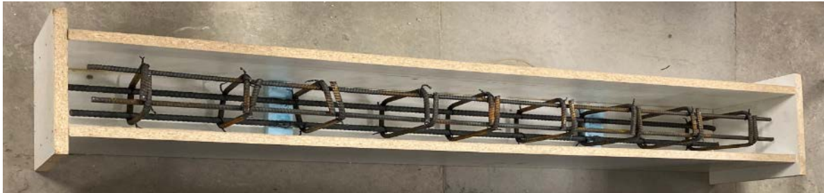
Figure 25. The Molds for Samples and Rebars before Casting of Concrete.
