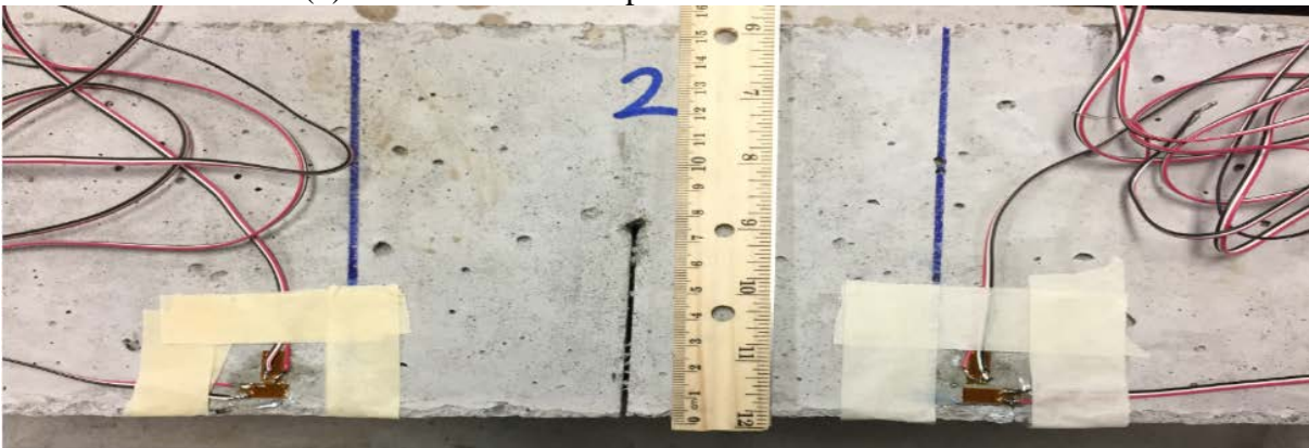
(c) Concrete beam sample with initial crack 25mm
