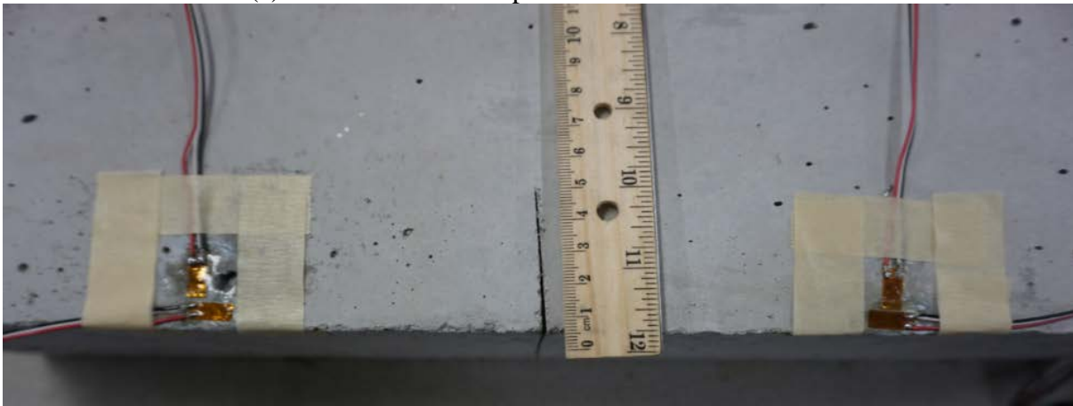
(b) Concrete beam sample with initial notch 50mm
