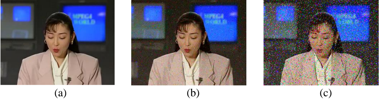
Figure 4. Video Output Example for s_{total} = 9.6 from Table 3., Numerical Example 1 ( V_{DD} = 0.75V ): (A) Original Video; (B) Video Stored by the Optimal Memory Design; (C) Video Stored by the Traditional Memory Design.
