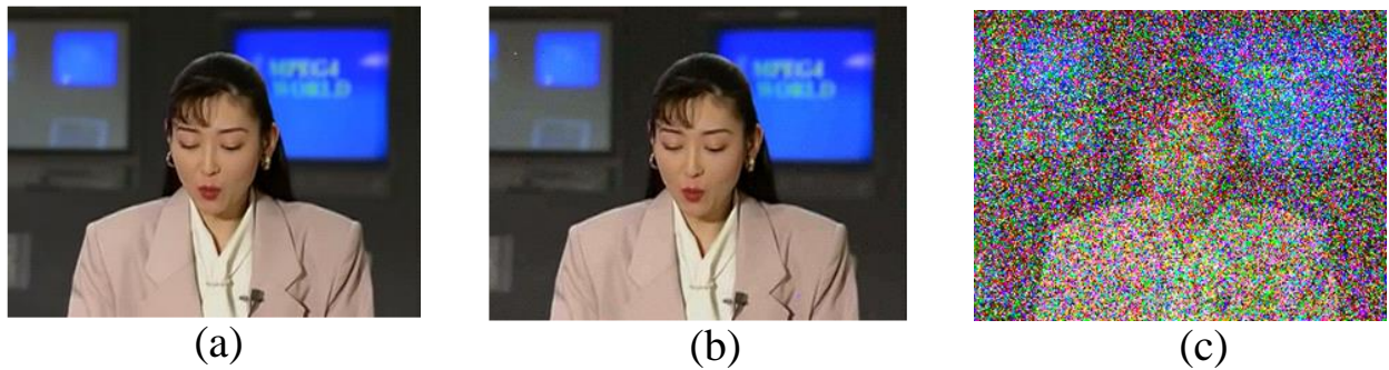
Figure 7. Video Output Quality Example for s_{total} = 8.7 from Table 5, Numerical Example 2 ( V_{DD} = 0.5V ): (A) Original Video; (B) Video Stored by the Optimal Design; (C) Video Stored by the Traditional Design.
