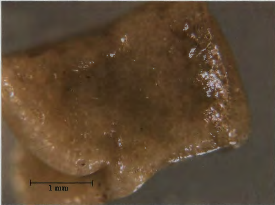
Figure 4.6 Biofilm formation on the surface of entrapment media at high HRT.
