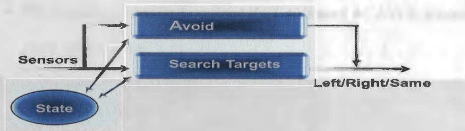
Figure 18. Subsumption Control Scheme for CUAV
