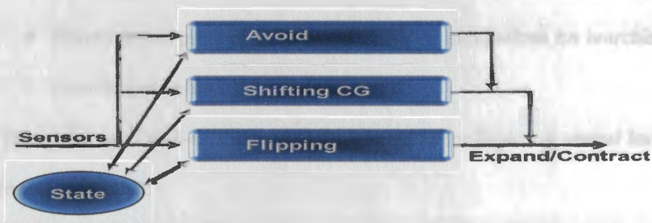
Figure 23. Modified Subsumption Control Scheme for Tetwalkers
