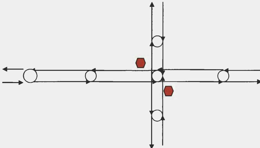
Figure 4.1. Link-Node Diagram in CORSIM<sup>®</sup> for 4-Legged Intersections.
