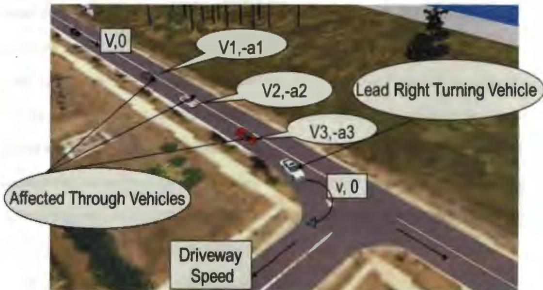
Figure 2.2. Impact on Through Vehicles due to Right-Turning Vehicles.
