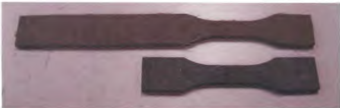
Figure 25: Extended tensile specimen.
