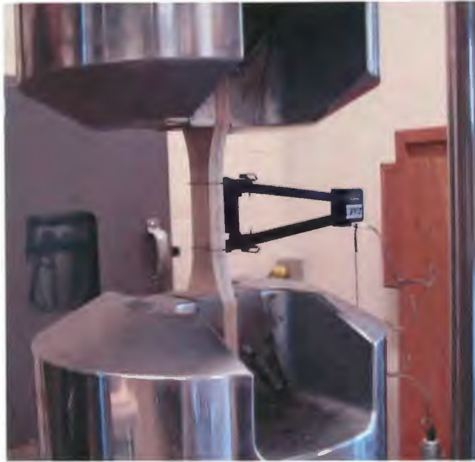
Figure 23: Tensile test with extensometer.
