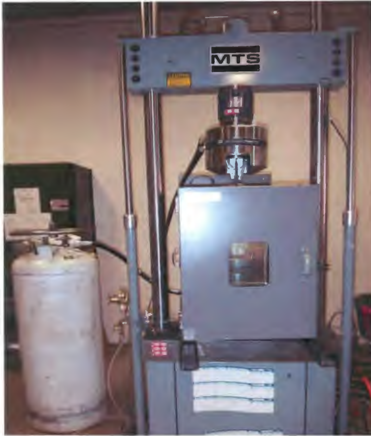
Figure 24: MTS load frame with environmental chamber.
