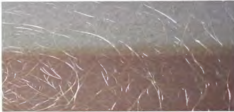
Figure 45: Discoloration as a result of UVA exposure.
