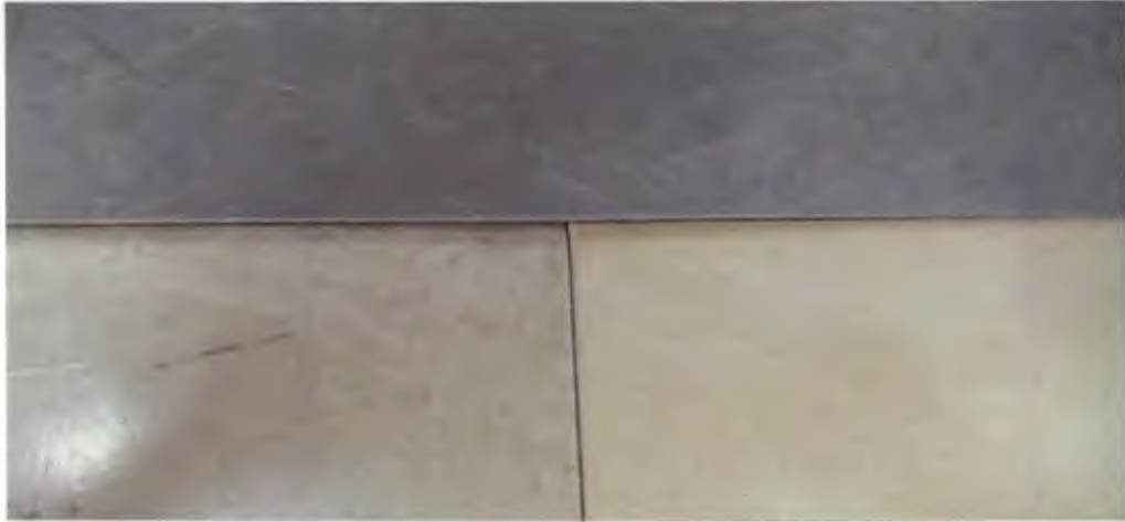
Figure 27: Set of the unconditioned processed panels; Top: carbon black filled, Bottom Left: sunflower filled, Bottom Right: neat PU.
