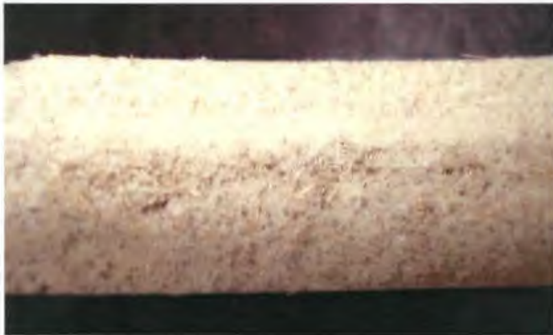
Figure 52: 20% by weight sunflower filler distribution.
