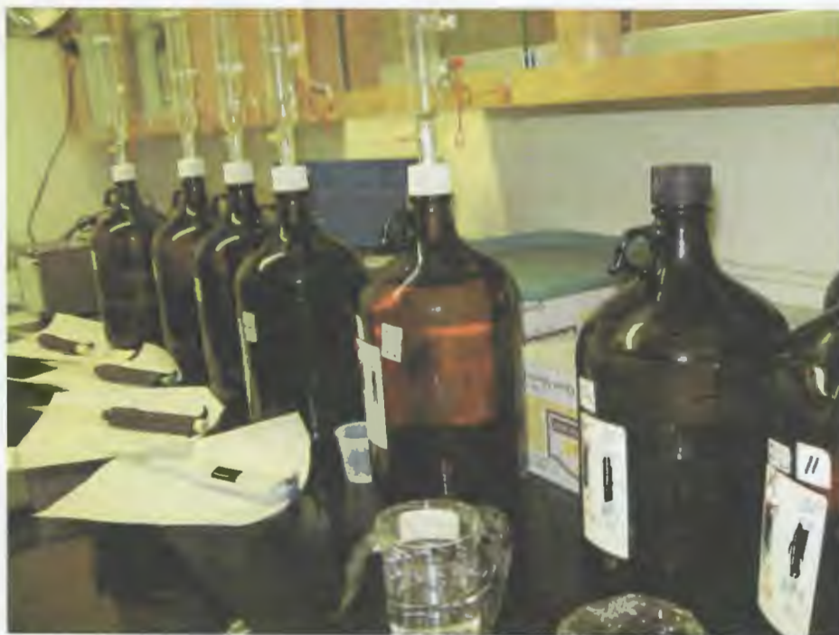
Fig. 26. Photograph of stock salt solutions (right) and ultra pure water containers fitted with repipette dispensers (middle). The pipettes in front of the water bottles were used to add the salt solution to the samples (left).
