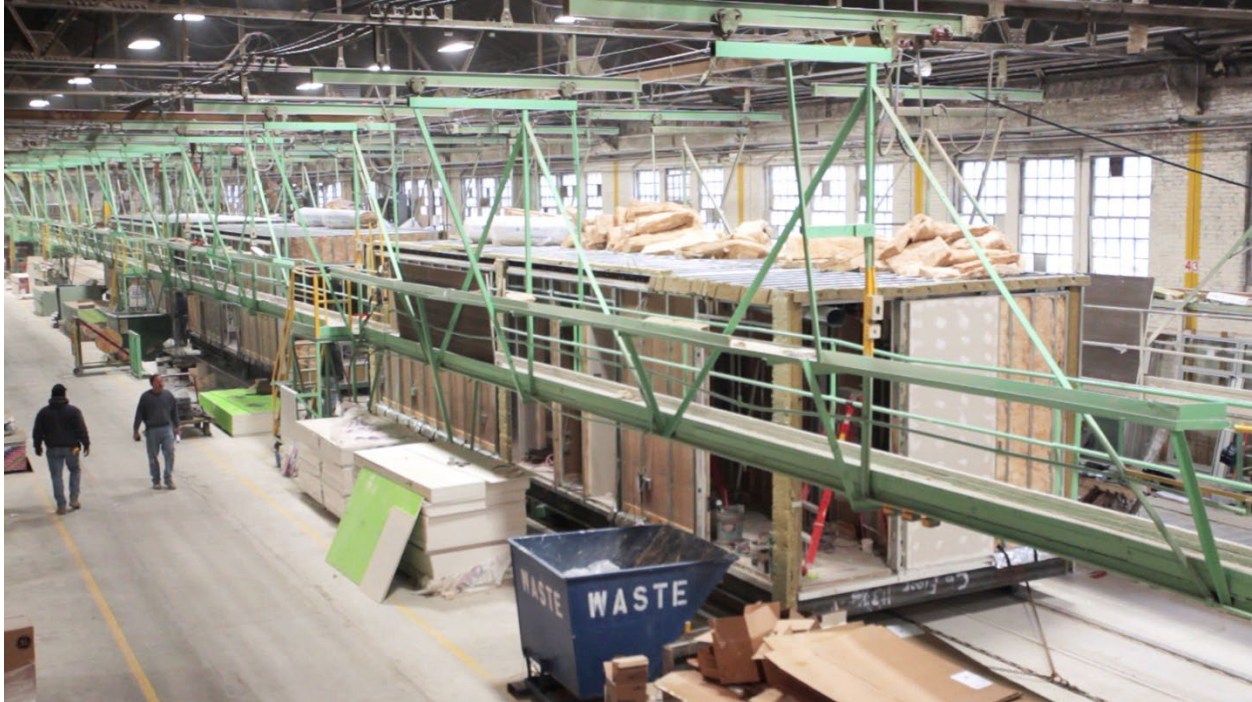
Figure 48. Image of the controlled industrial environment in which the individual modules of The Stack NYC were fabricated. Credit: GLUCK+
