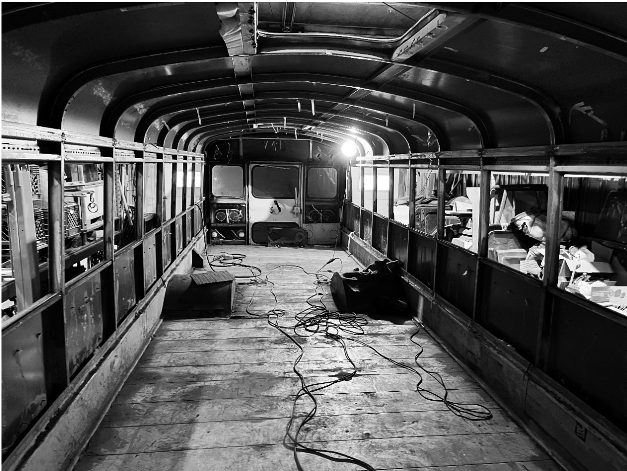
Figure 3.3.3.2 Framing of School Bus
