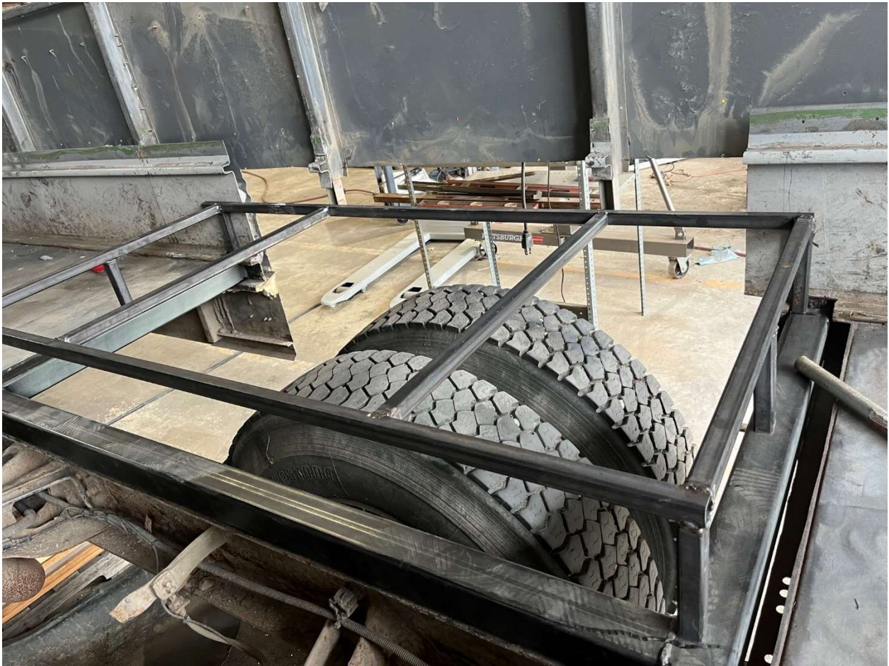
Figure 4.3.2.8 Steel Framing of Wheel Well
