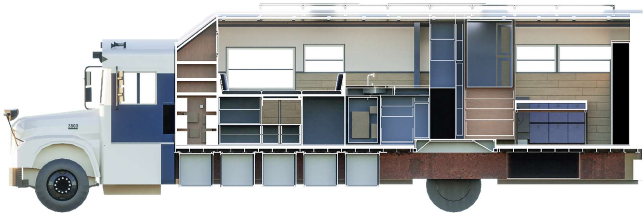
Figure 4.4.2.6 Driver's Side Section
