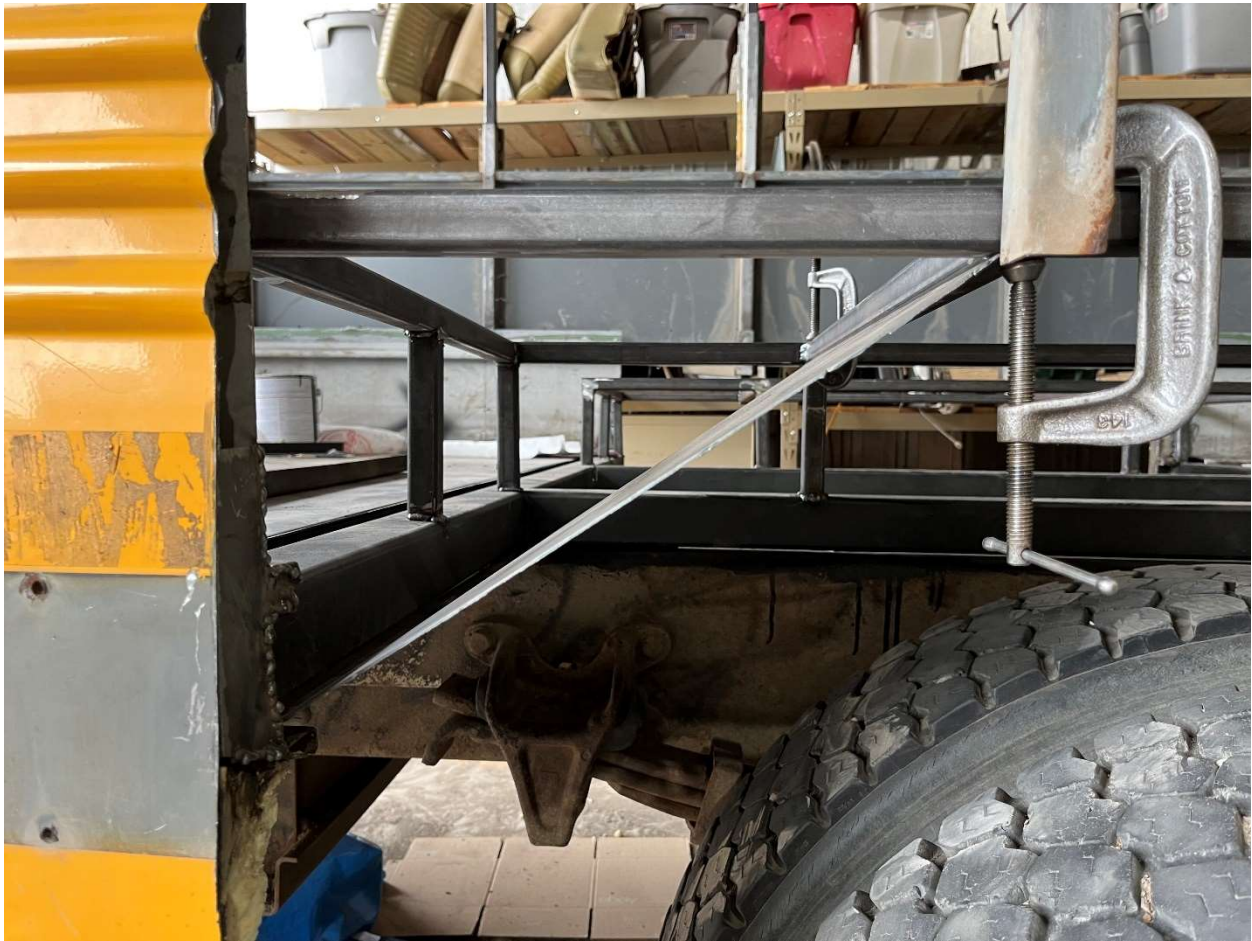
Figure 4.3.2.9 Sheet Metal Attached to Framing
