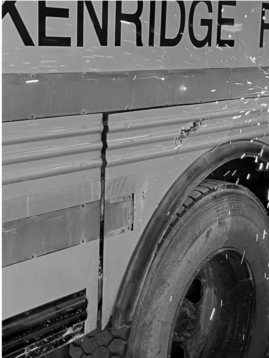
Figure 2.3.1 Rust Hole in Exterior of School Bus
