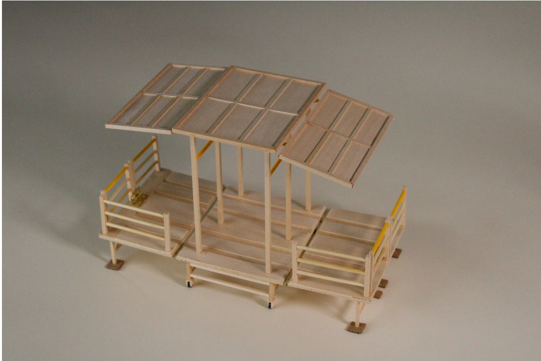
Figure 4.12. "Seattle Pavilion Section Physical Model."
