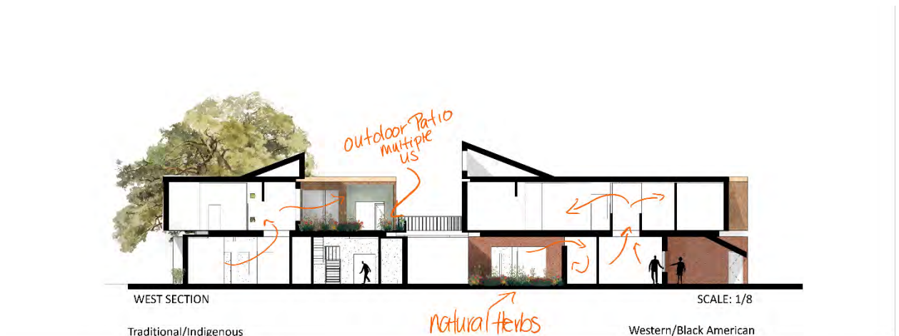
Figure 20 Westside section cut w/ illustration of air flow with aromatic oils herbs and location of African traditional herbs
