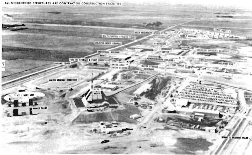
Fig 3. Picture of the Stanley R Mickelsen Defense Complex, Contained in A History of the Huntsville Division, U.S. Army Corp of Engineers 1967-1976 .
