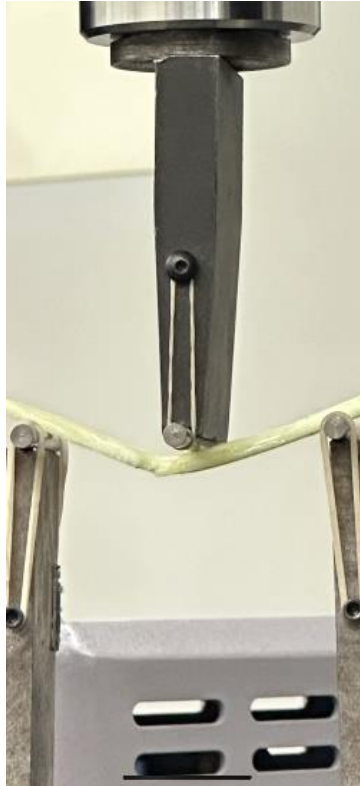
Figure 27: PX composite bending under flexural load.
