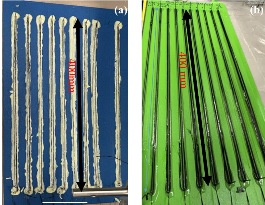
Figure 6: Composite samples printed with (a) PX, and (b) Epon-Epikure resin system.
