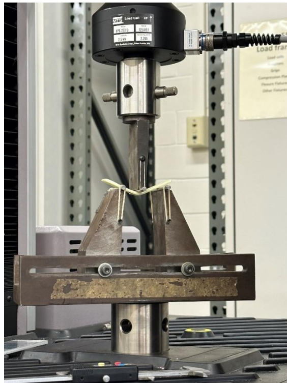
Figure 14: 3-point bend test setup.
