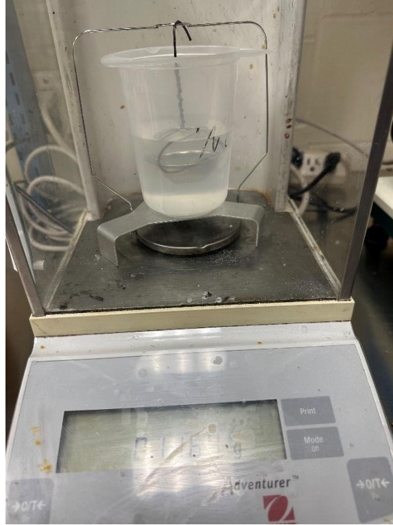
Figure 11: Density test setup for composite printed specimen.
