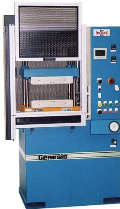
Figure 6. Wabash Genesis four-post compression press [25]
