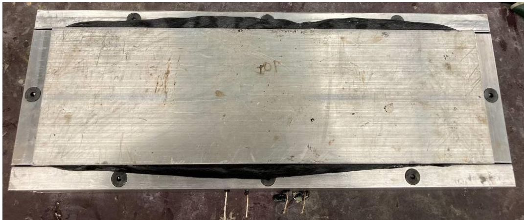
Figure 21. Post-processed mold showing polymer and fiber flashing
