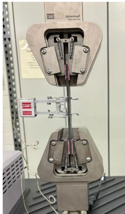
Figure 10. 0° tensile test with extensometer
