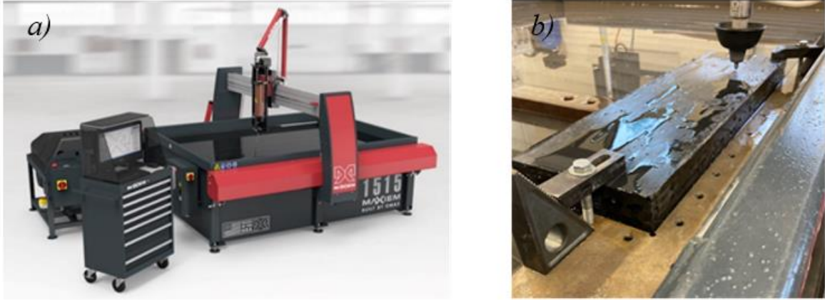
Figure 14. a) Maxiém 1515 waterjet [29] and b) waterjet cutting 2 in sample
