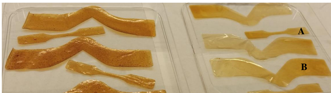
Figure 3.3. AX Films cutting by tear and tensile dies. A: tensile shape. B: tear shape.
