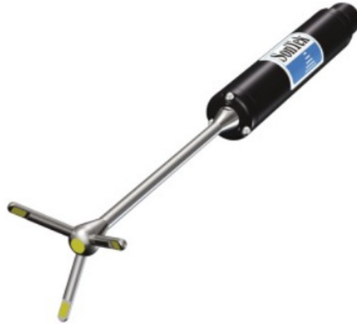
Figure 1.3. 10 MHz Sontek ADV (Neill & Hashemi, 2018).
