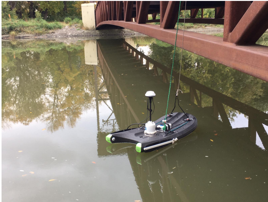
Figure 1.4. Hydroboard-mounted ADCP, Sontek M9, during the Fall measurements of 2020.
