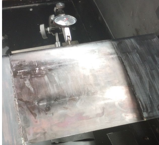
Figure 20. Dial indicator test setup within the wind tunnel.
