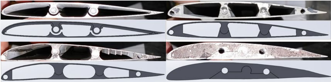
Figure 5. Comparison of the models as-built vs. drawn.
