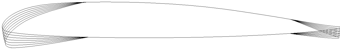
Figure 6. XFLR 5 variation of leading and trailing edged deflections of a VR-12 airfoil. [24]
