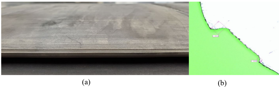
Figure 16. Photography of leading edge with microcavity (a) and microscope image detail of the microcavity cross section (b).
